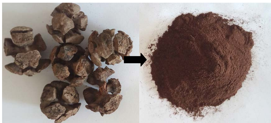
Fig. 1. Raw and grinded (60–120 \mu\text{m} particle size) forms of low-cost bioadsorbent CCS.
