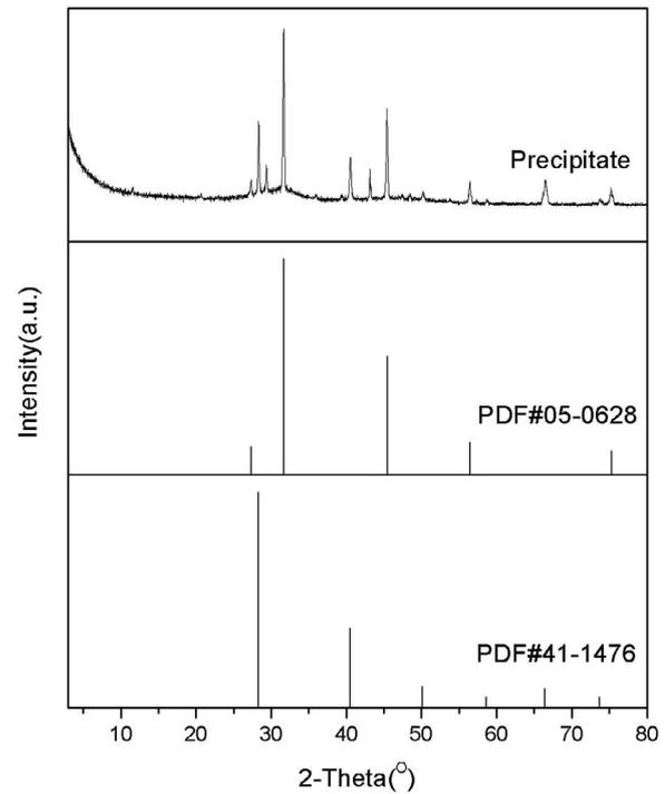
Fig. S6. XRD pattern of the precipitate collected from the formulation based on the composition of *S. spectabile*'s roots cultivated in culture medium B with NaCl stress (third column in Table S7) (PDF#05-0628 Halite ( $\text{NaCl}$ ), syn; PDF#41-1476 Sylvite ( $\text{KCl}$ ), syn).
