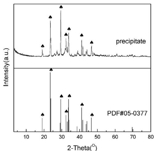
Fig. 4. XRD pattern of a precipitate obtained from a potassium nitrate solution at 15°C.
