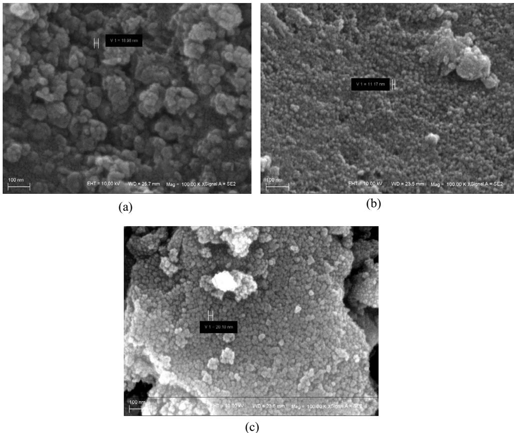
Fig. S10. SEM photomicrographs of the floccules: (a) calcium phosphate floccules, (b) Al-containing floccules, and (c) Fe-containing floccules.
