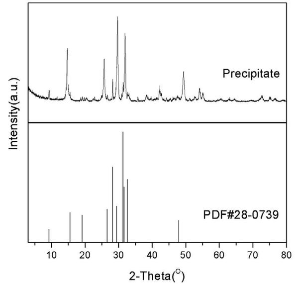
Fig. S9. XRD pattern of the precipitate collected from the formulation based on the composition of *S. spectabile*'s roots cultivated in culture medium B with  $\text{Na}_2\text{SO}_4$  stress (third column in Table S7, except without addition of  $\text{KH}_2\text{PO}_4$ ) [PDF#28-0739 Syngenite ( $\text{K}_2\text{Ca}(\text{SO}_4)_2 \cdot \text{H}_2\text{O}$ ), syn].
