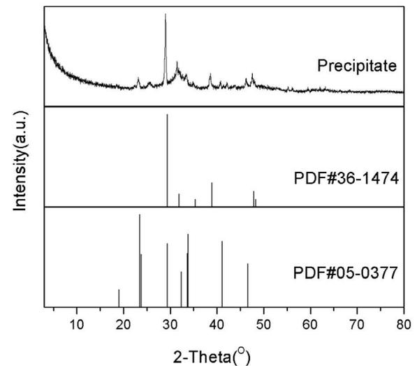
Fig. S7. XRD pattern of the precipitate collected from the formulation based on the composition of *S. spectabile*'s roots cultivated in culture medium B with  $\text{NaNO}_3$  stress (third column in Table S8) (PDF#36-1474 Nitratine ( $\text{NaNO}_3$ ), syn; PDF#05-0377 Niter ( $\text{KNO}_3$ ), syn).
