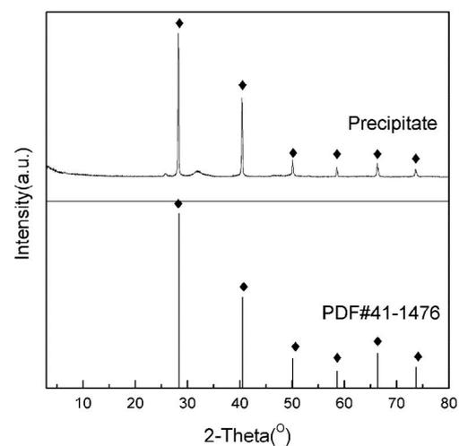
Fig. 2. XRD pattern of a precipitate obtained from a potassium chloride solution at 15°C.
