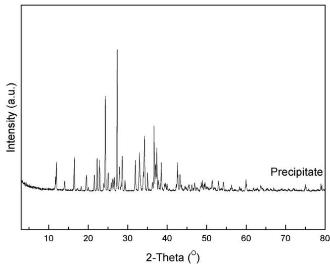
Fig. S5. XRD pattern of the precipitate collected from KCl,  $\text{KNO}_3$ , or  $\text{K}_2\text{SO}_4$  solution with tartaric acid.
