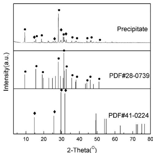
Fig. 5. XRD pattern of a precipitate collected from a potassium sulfate solution.
