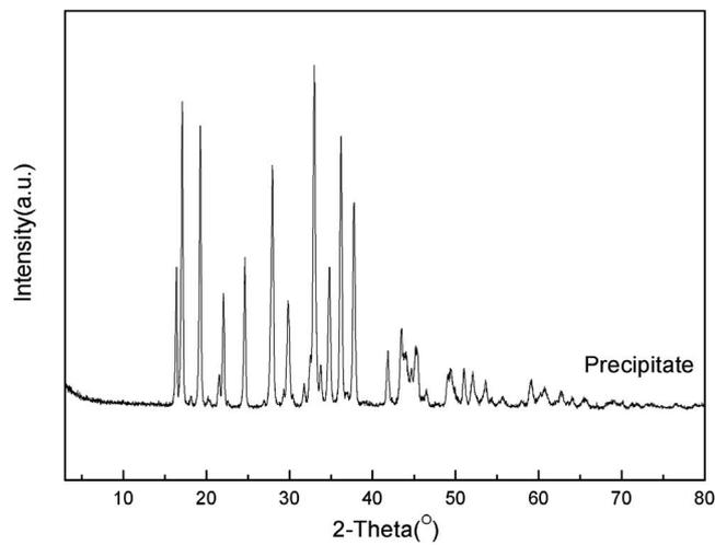
Fig. S4. XRD pattern of the precipitate collected from NaCl,  $\text{NaNO}_3$ , or  $\text{Na}_2\text{SO}_4$  solution with oxalic acid.
