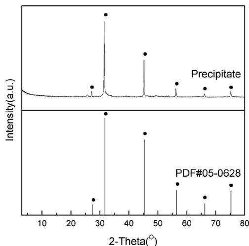
Fig. 1. XRD pattern of a precipitate obtained from a sodium chloride solution at 15°C.
