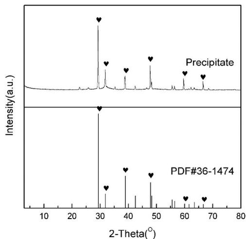
Fig. 3. XRD pattern of a precipitate obtained from a sodium nitrate solution at 15°C.
