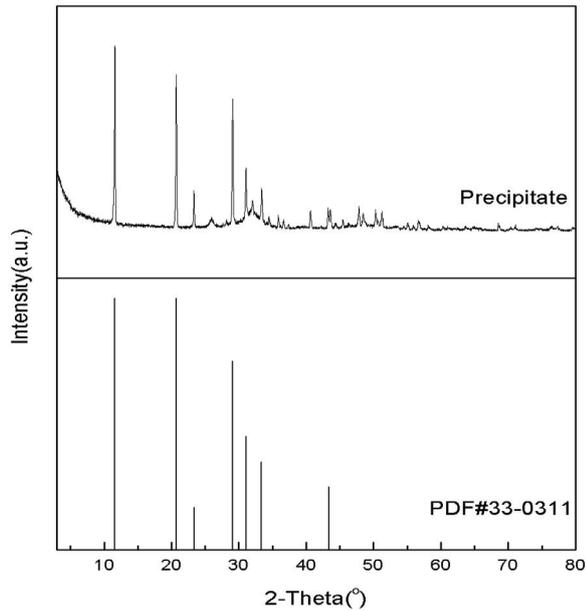
Fig. S8. XRD pattern of the precipitate collected from the formulation based on the composition of *S. spectabile*'s roots cultivated in culture medium B with  $\text{Na}_2\text{SO}_4$  stress (third column in Table S9) [PDF#33-0311 Gypsum ( $\text{CaSO}_4 \cdot 2\text{H}_2\text{O}$ ), syn].
