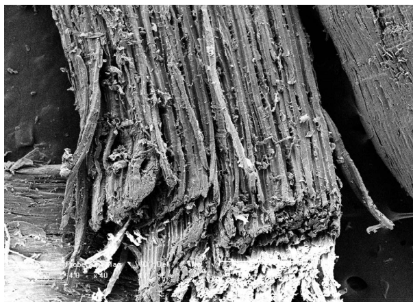
Fig. 4. Surface characterization of wood particles in a SEM photomicrograph (40X) (a) and with scanning electron EDS (b).
