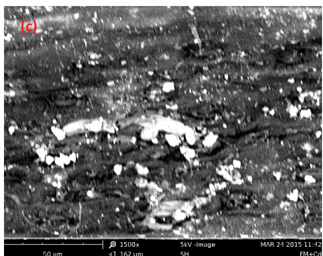
Fig. 3. SEM micrograph ( \times 1,500 ) of CL before (a) and after (b) copper and (c) cadmium biosorption.
