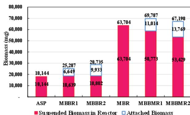
Fig. 10. Comparison of biomass in different operation.
