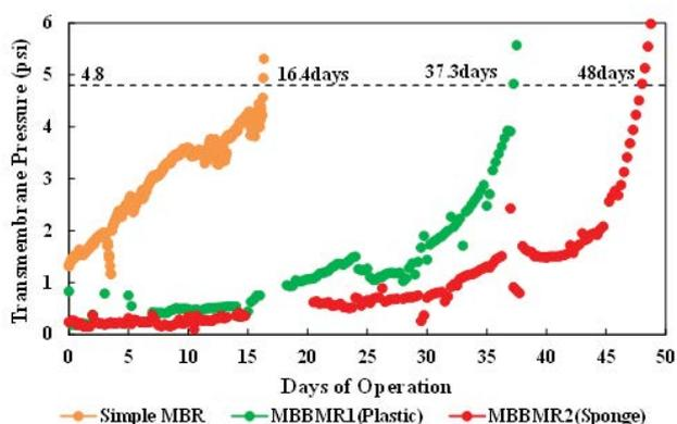
Fig. 9. TMP profile of simple MBR, MBBMR1 and MBBMR2.
