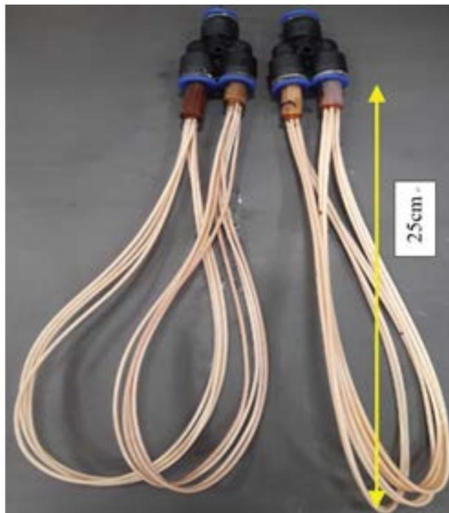
Fig. 2. Membrane module used in MBR and MBBMR.
