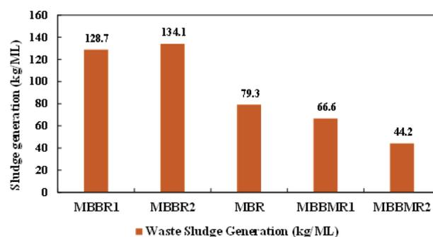
Fig. 12. Waste sludge generation of different technologies.
