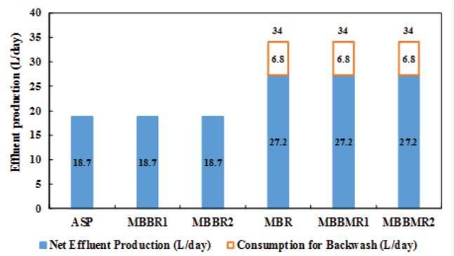
Fig. 8. Effluent production of all different technologies.
