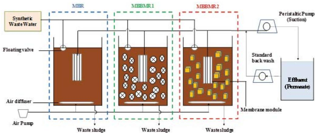
Fig. 4. Schematic diagram of MBR and MBBMR plants.
