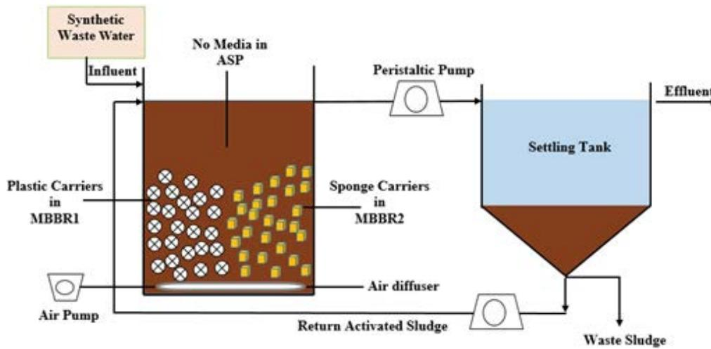
Fig. 3. Schematic diagram of ASP and MBBR plants.
