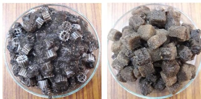
Fig. 11. Attached biomass on the plastic and sponge carriers.
