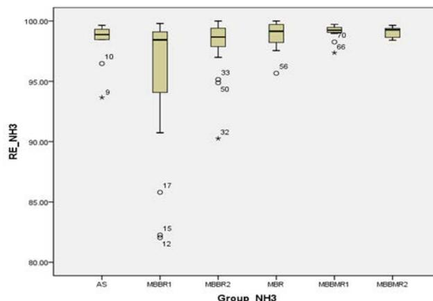
Fig. 7. Distribution of removal efficiency of  $\text{NH}_4^+\text{-N}$  across all operations.
