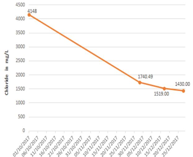
Fig. 2. Reduction of chloride by Reeds roots.
