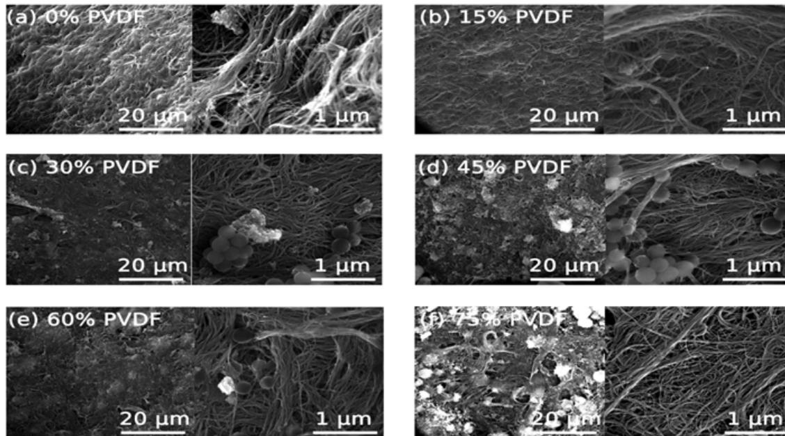
Fig. 5. SEM photos of CNT membranes.
