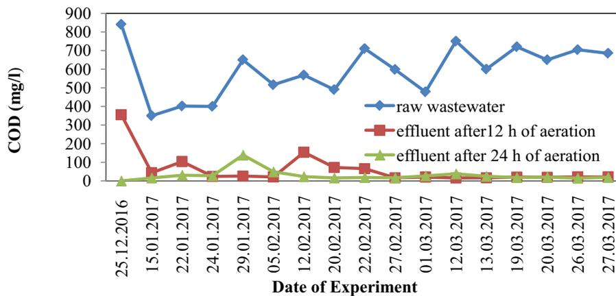
Fig. 5. COD in wastewater and effluents after 12 and 24 h of aeration at DO 4 mg/L.
