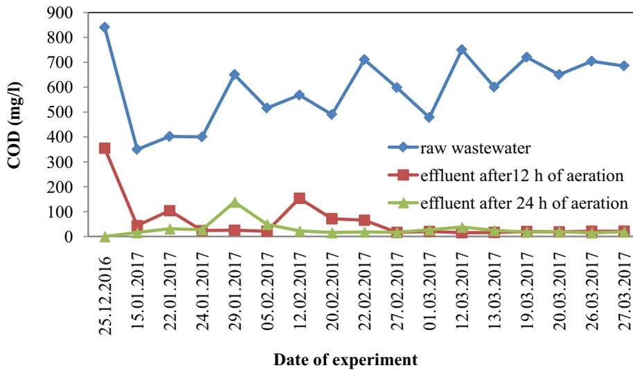
Fig. 4. COD in wastewater and effluents after 12 and 24 h of aeration at DO 2 mg/L.
