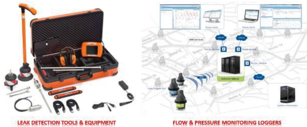
Fig. 8. Used leak detection tools and softwares.
