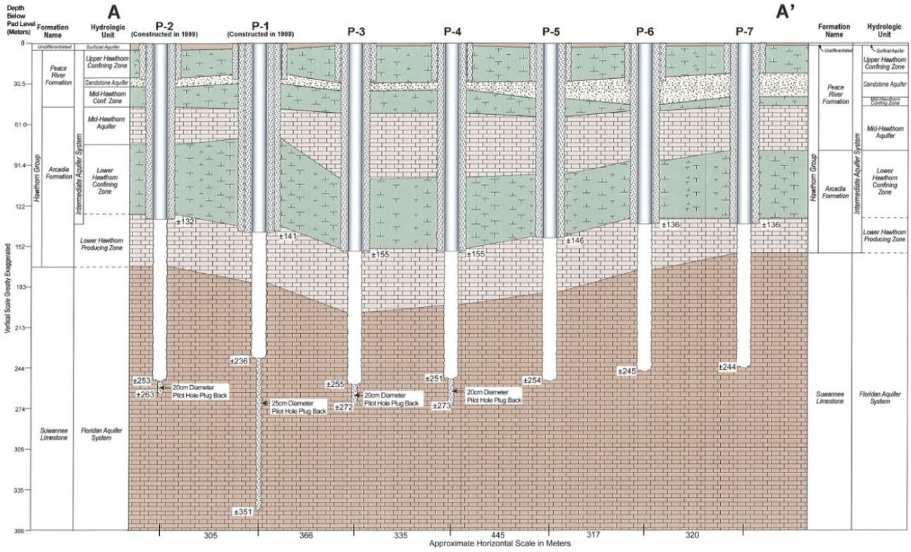
Fig. 3. North-south geological cross-section through wells P-1 to P-7 in the City of Fort Myers, Florida wellfield [11].
