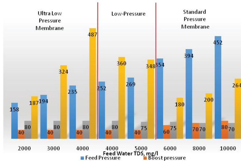
Fig. 11. Brackish water membrane options based on increasing feed water TDS and the impact on permeate quality, membrane feed pressure, and recovery (Missimer et al. [5]).
