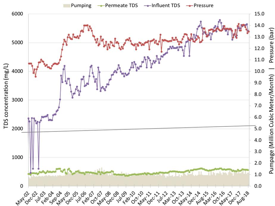
Fig. 10. Diagram showing monthly pumpage, influent and permeate TDS concentrations, and membrane operating pressure.
