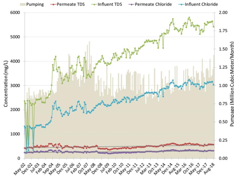
Fig. 9. Diagram showing monthly pumpage, influent and permeate concentrations of TDS and dissolved chlorides. The BWRO process in the plant has been adjusted to produce permeate that consistently meets drinking water standards.
