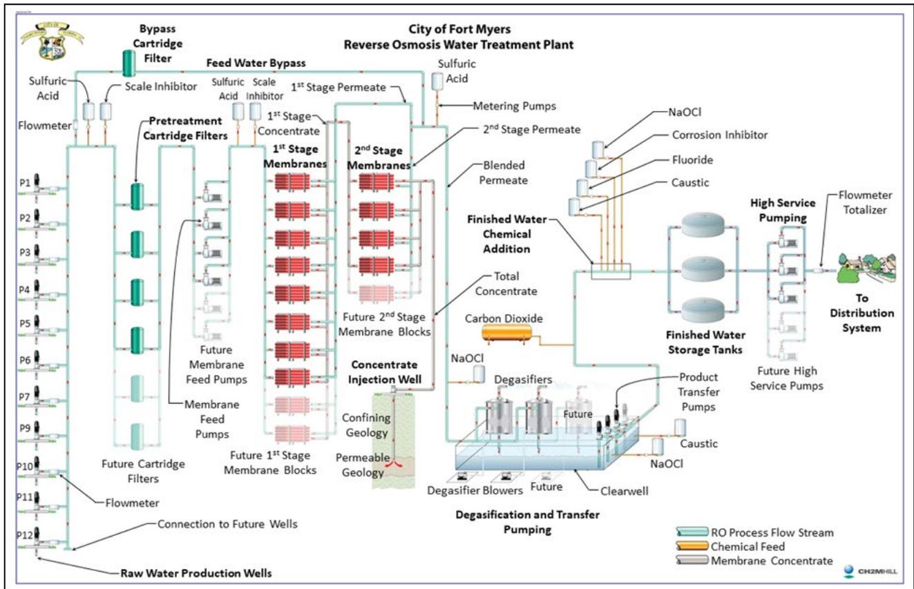
Fig. 6. Process flow diagram for the City of Fort Myers RO water treatment facility.
