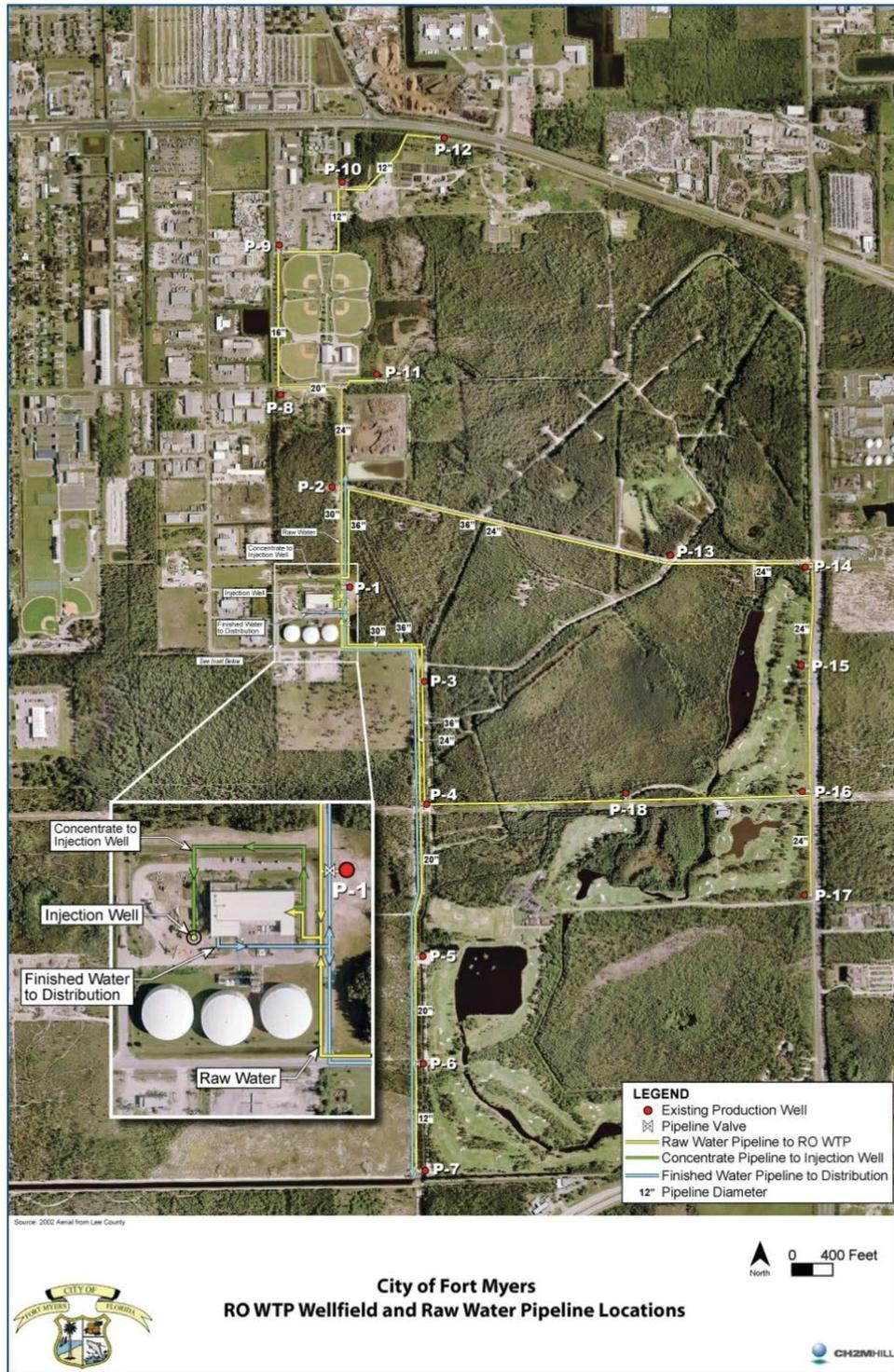
Fig. 2. Map of the City of Fort Myers RO water treatment facility and the production wells used to supply feed water.
