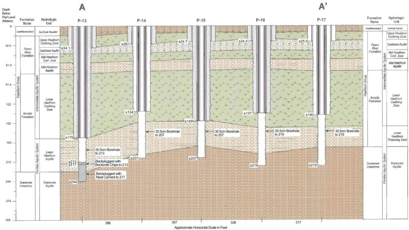
Fig. 4. North-south geological cross-section through wells P-13 to P-17 in the City of Fort Myers, Florida wellfield [12].
