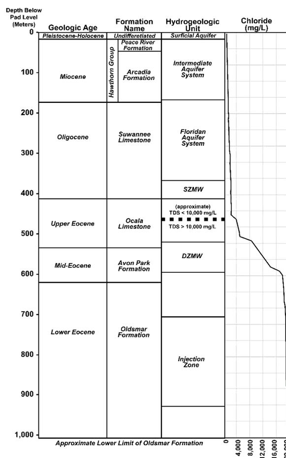
Fig. 5. The geological section of the injection well located at the City of Fort Myers wellfield with water quality in each aquifer penetrated (modified from CH2MHill [13]). Note that there is considerable inaccuracy in these data in that they conflict with the data from well P-1 which is located close to the injection well site.
