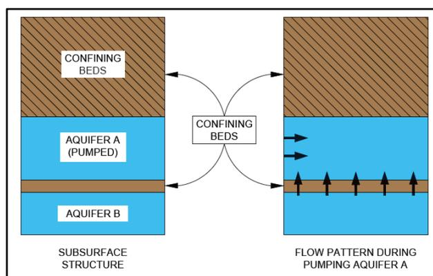
Fig. 1. Diagram showing upward recharge of an aquifer containing brackish-water during pumping (Missimer [2]).
