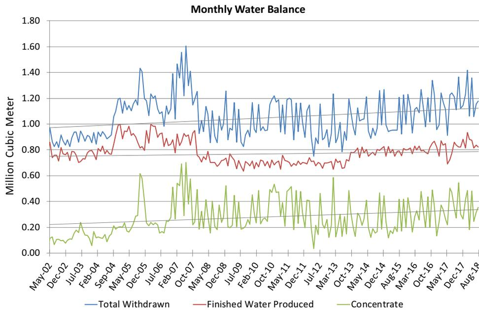
Fig. 7. Monthly water balance showing the total water withdrawn, finished water produced, and the treatment losses.
