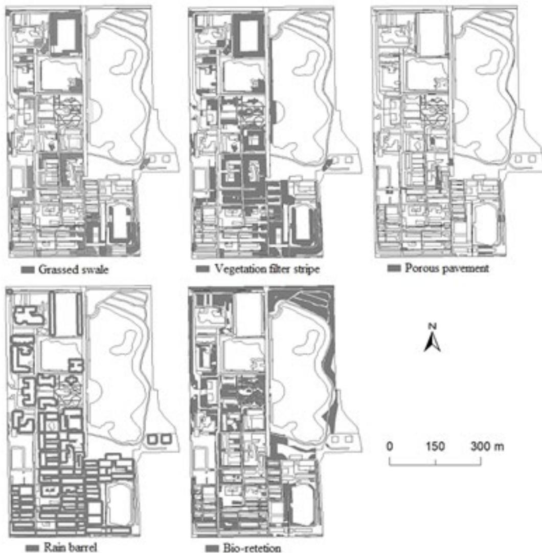
Fig. 2. Suitable positions and types of LID facilities.
