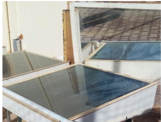
Fig. 3. Distiller D2 with a refractor.
