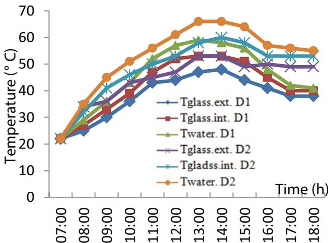
Fig. 5. Evolution of the inner glazing temperature of the distillers.
