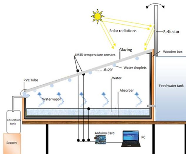
Fig. 2. Croquet of the solar still with a refractor.
