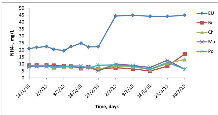
Fig. 10. Variations of  $\text{NH}_4\text{-N}$  for different MSL-column systems (EU): raw wastewater, (Br): MSL reference, (Ch): charcoal, (Ma): marble waste, and (Po): pozzolan.
