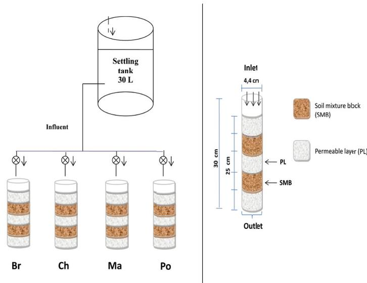
Fig. 1. Laboratory-scale MSL systems: (Br): MSL reference, (Ch): charcoal, (Ma): marble waste, and (Po): pozzolan.
