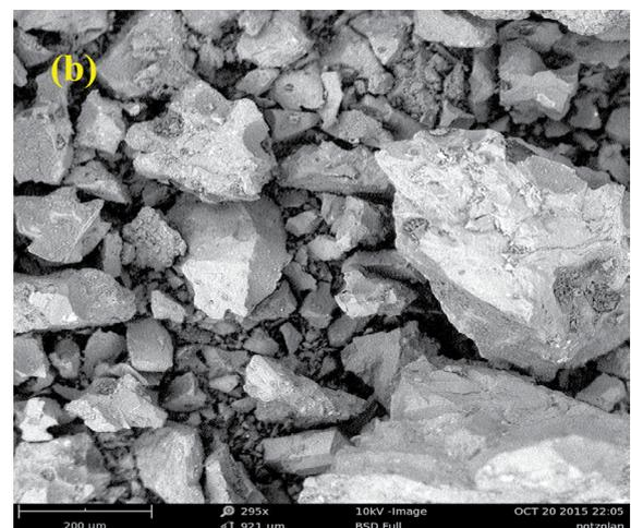
Fig. 2. SEM images of powdered marble at 100 mm (a) and pozzolan (b) at 200 mm.
