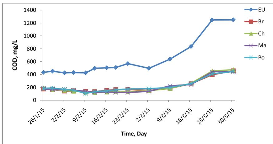
Fig. 7. Variations of COD for different MSL-column systems (EU): raw wastewater, (Br): MSL reference, (Ch): charcoal, (Ma): marble waste, and (Po): pozzolan.
