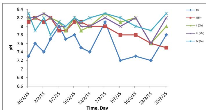
Fig. 4. Variation of the pH for different MSL-column systems (EU): raw wastewater, (Br): MSL reference, (Ch): charcoal, (Ma): marble waste, and (Po): pozzolan.
