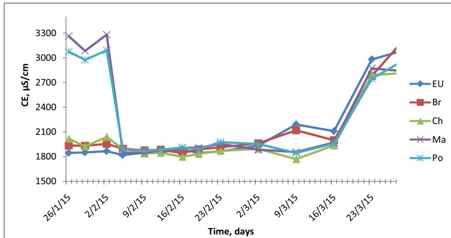
Fig. 5. Variations of electrical conductivity for different MSL-column systems (EU): raw wastewater, (Br): MSL reference, (Ch): charcoal, (Ma): marble waste, and (Po): pozzolan.
