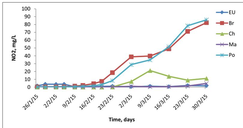
Fig. 11. Variations of  $\text{NO}_2\text{-N}$  for different MSL-column systems (EU): raw wastewater, (Br): MSL reference, (Ch): charcoal, (Ma): marble waste, and (Po): pozzolan.
