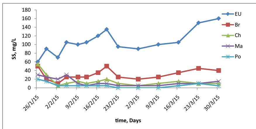
Fig. 8. Variations of SS for different MSL-column systems (EU): raw wastewater, (Br): MSL reference, (Ch): charcoal, (Ma): marble waste, and (Po): pozzolan.
