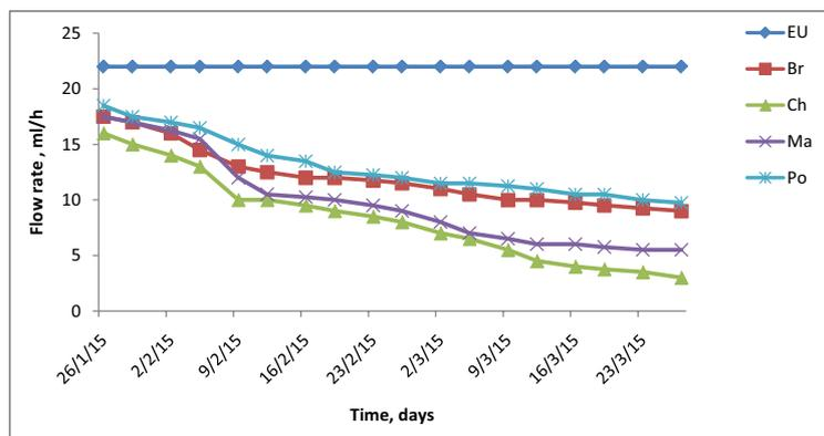
Fig. 3. Flow rate for different MSL-column systems (EU): raw wastewater, (Br): MSL reference, (Ch): charcoal, (Ma): marble waste, and (Po): pozzolan.
