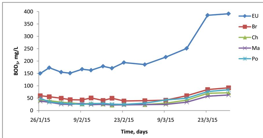
Fig. 6. Variations of BOD<sub>5</sub> for different MSL-column systems (EU): raw wastewater, (Br): MSL reference, (Ch): charcoal, (Ma): marble waste, and (Po): pozzolan.
