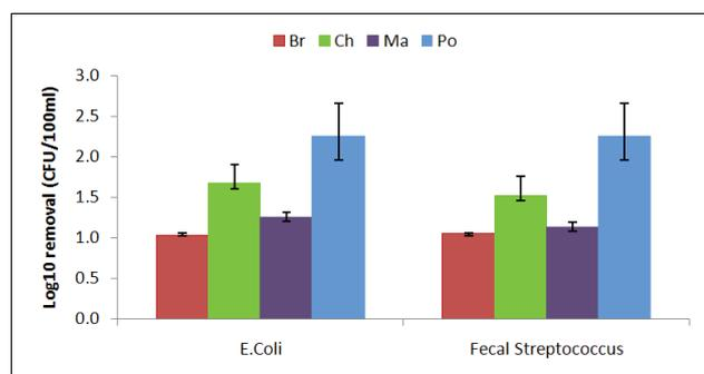
Fig. 12. Average removal efficiencies of bacterial indicators with different materials (EU): raw wastewater, (Br): MSL reference, (Ch): charcoal, (Ma): marble waste, and (Po): pozzolan.
