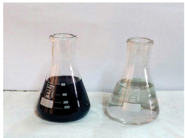
Fig. 13. AC-ZnO composite performance in real sewage.
