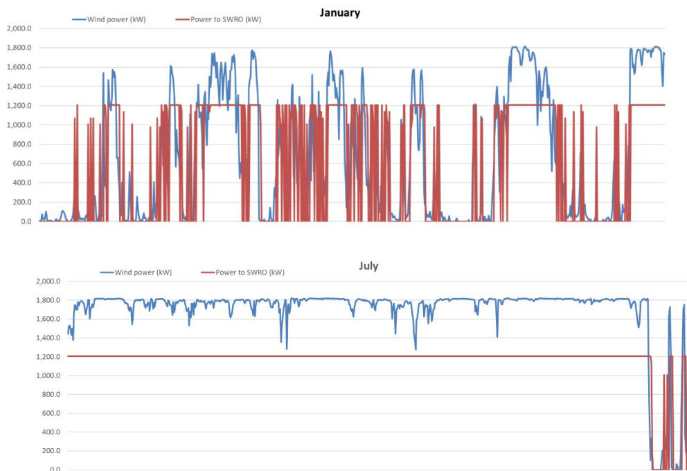
Fig. 5. Case 1.a Wind and batteries coupled to a conventional SWRO plant.
