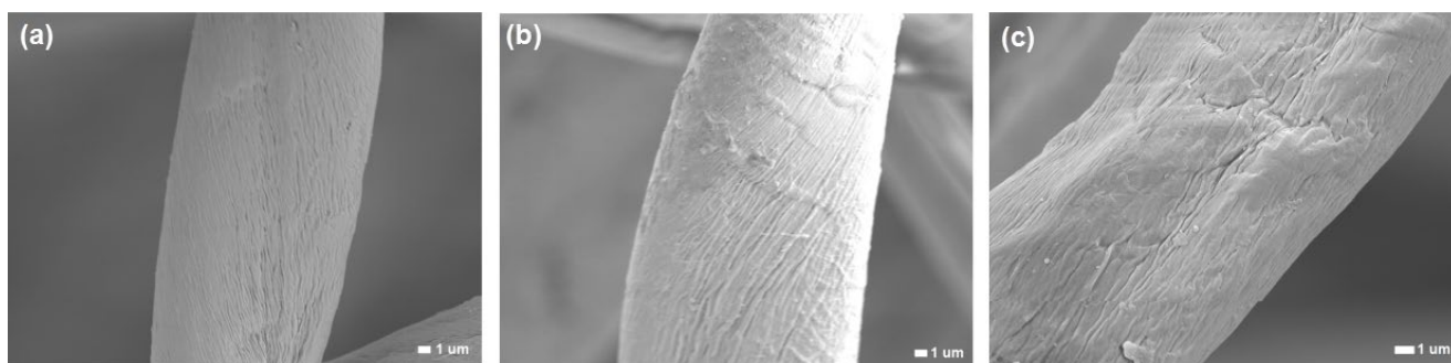
Fig. 2. SEM images of the degreasing cotton (a), ADC (b) and HA-adsorbed ADC (c).
