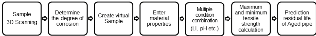
Fig. 2. Modified process for the prediction of residual life of aged pipe through tensile strength simulation and conventional method.
