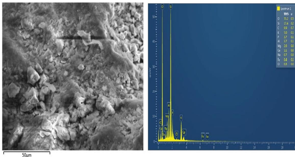
Fig. 2. SEM image and EDX graph taken under optimum conditions using MAP precipitation method in leachate.
