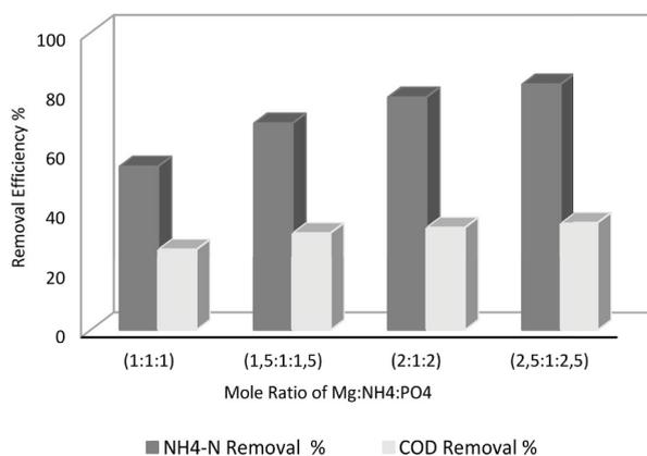
Fig. 7. Ammonia and COD removal efficiencies at different molar ratio of Mg and PO<sub>4</sub>.
