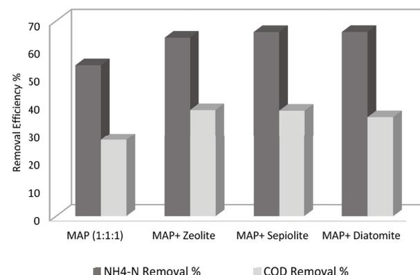
Fig. 8. Effect of adding natural materials to MAP precipitation process on ammonia and COD removal.
