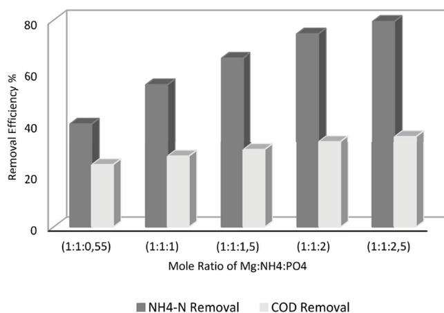
Fig. 6. Ammonia and COD removal efficiencies at different molar ratio of PO<sub>4</sub>.
