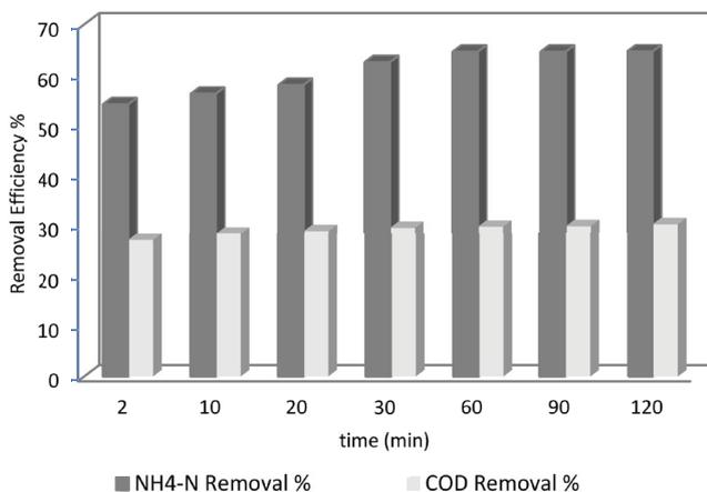
Fig. 4. Effect of stirring time on ammonia and COD removal efficiency.
