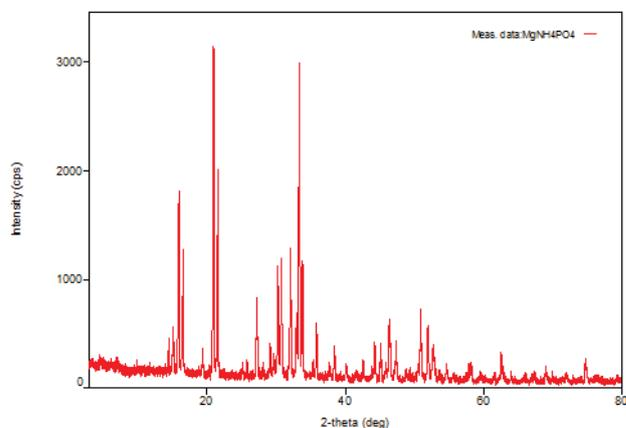
Fig. 1. XRD graph of leachate using MAP precipitation method under optimum conditions.
