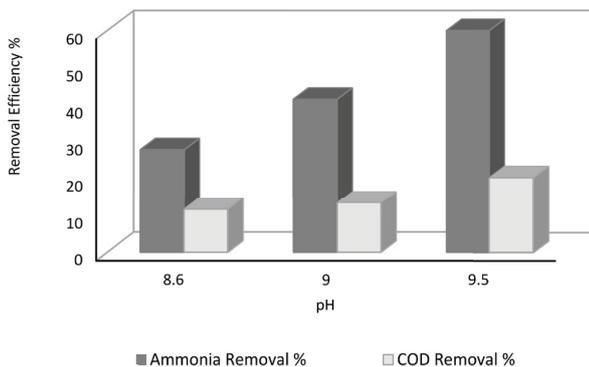
Fig. 3. Effect of initial pH on removal efficiency ( $\text{Mg}:\text{NH}_4:\text{PO}_4$  molar ratio of 1:1:1).
