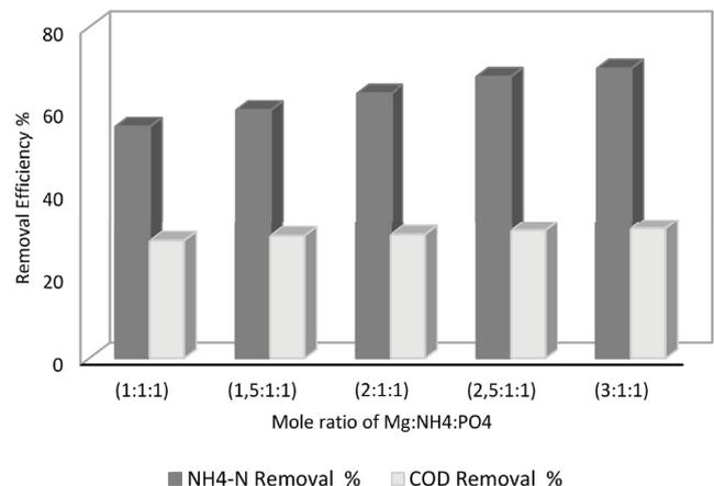
Fig. 5. Ammonia and COD removal efficiencies at different molar ratio of Mg.
