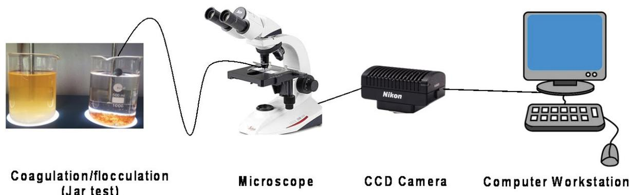
Fig. 2. Illustration of the experimental setup used for image analysis of flocs.
