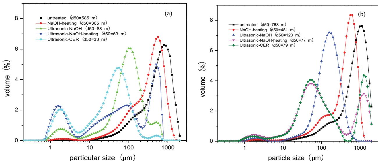
Fig. 3. Granulometric distribution by volume of untreated and four extracted sludge in R1 and R2.
