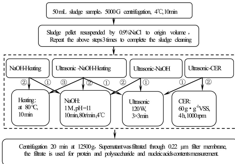
Fig. 1. Procedures for the EPS extraction protocols.
