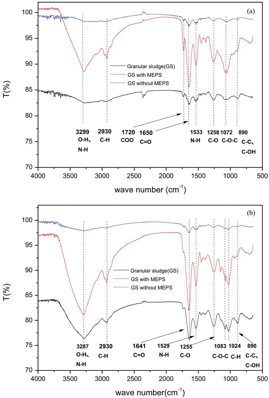
Fig. 5. Different Fourier-transform infrared spectra of granular sludge (GS), GS with MEPS and GS without MEPS in R1 and R2. Note: GS with MEPS was the granular sludge after the ultrasonic extraction, GS without MEPS was the granular sludge after ultrasonic-CER extraction.
