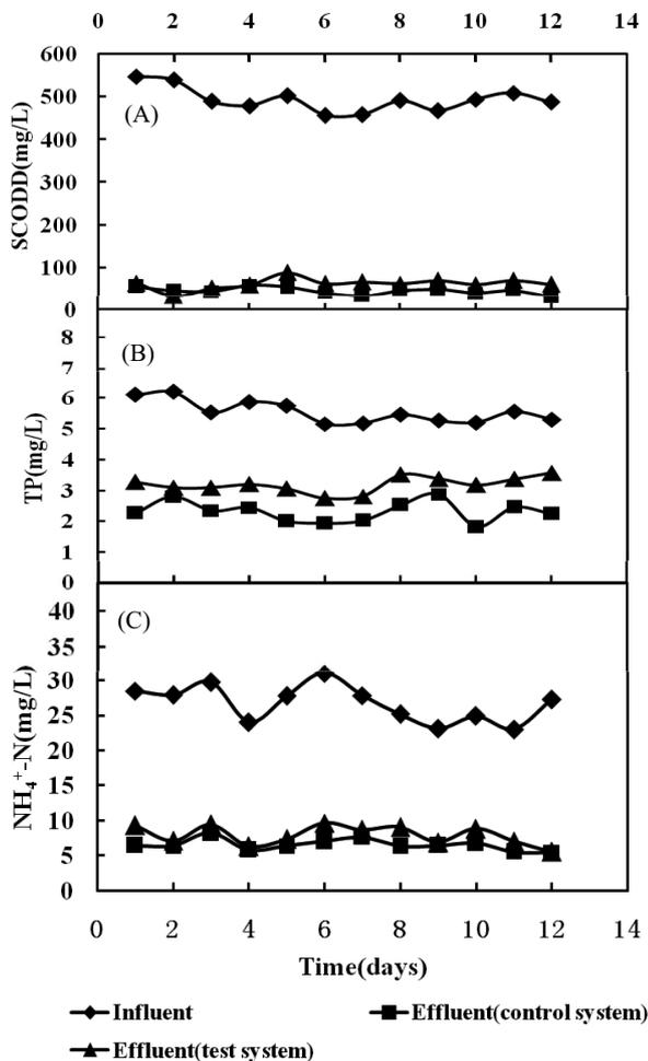
Fig. 5. Variations of the SCOD (a), TP (b) and  $NH_4^+-N$  (c) in the effluent of the control system and test system.
