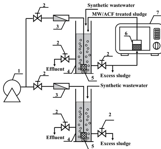
Fig. 1. Schematic illustration of MW/ACF-activated sludge process combined system: (1) air compressor; (2) manual valve; (3) flow meter; (4) SBR system; (5) micro-porous aerator; (6) Teflon vessel with ACF; (7) Microwave furnace.
