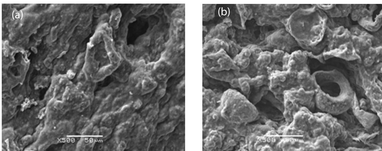
Fig. 3. SEM images of sludge before (a) and after MW/ACF pretreatment (b).
