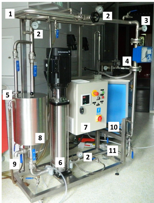
Fig. 1. Cross-flow filtration system: 1—water coat, 2—manometer, 3—thermometer, 4—flowmeter, 5—regulating valves, 6—high-pressure pump, 7—control box with an inverter, 8—tank, 9—drain from the tank, 10—membrane module, 11—permeate outlet.
