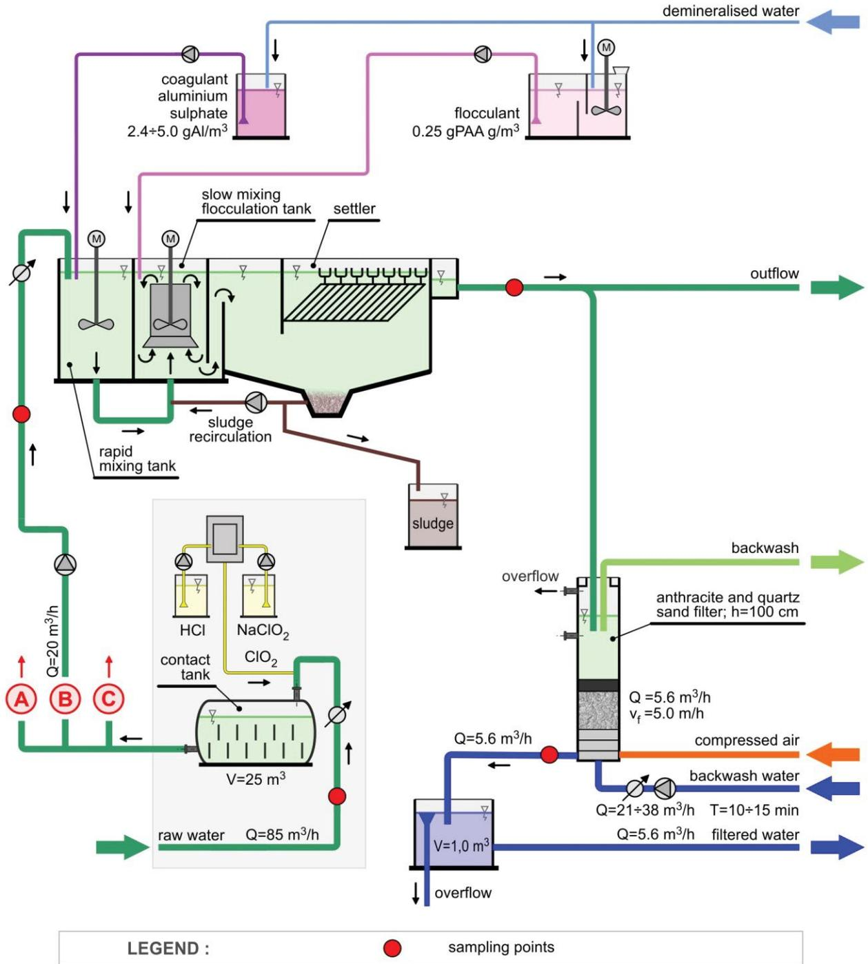
Fig. 2. Flow chart of the technological processes analyzed during the coagulation, sedimentation with sludge recirculation and filtration.
