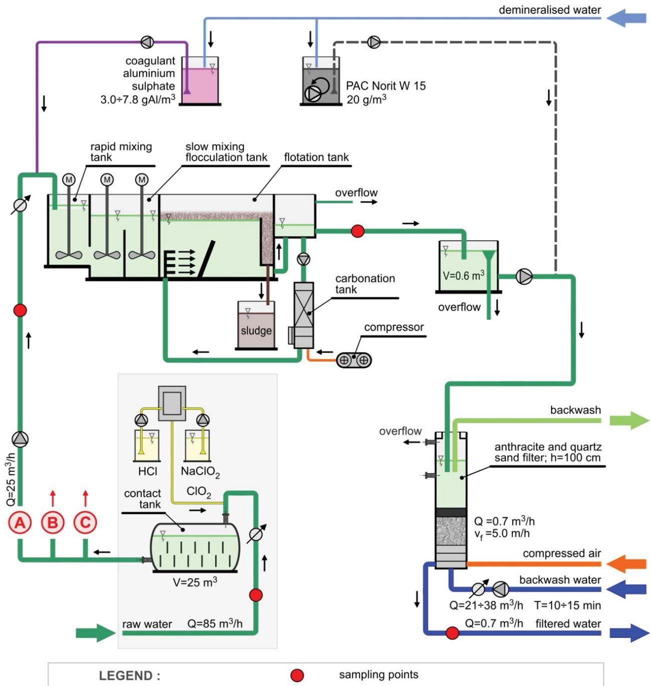
Fig. 1. Flow chart of the technological processes analyzed during the coagulation with sludge flotation and filtration.
