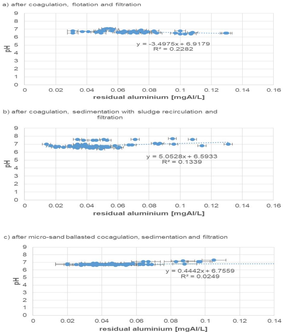
Fig. 5. Relationship between the concentration of the residual aluminium and the pH in the water after the coagulation, flotation or sedimentation, and filtration processes.
