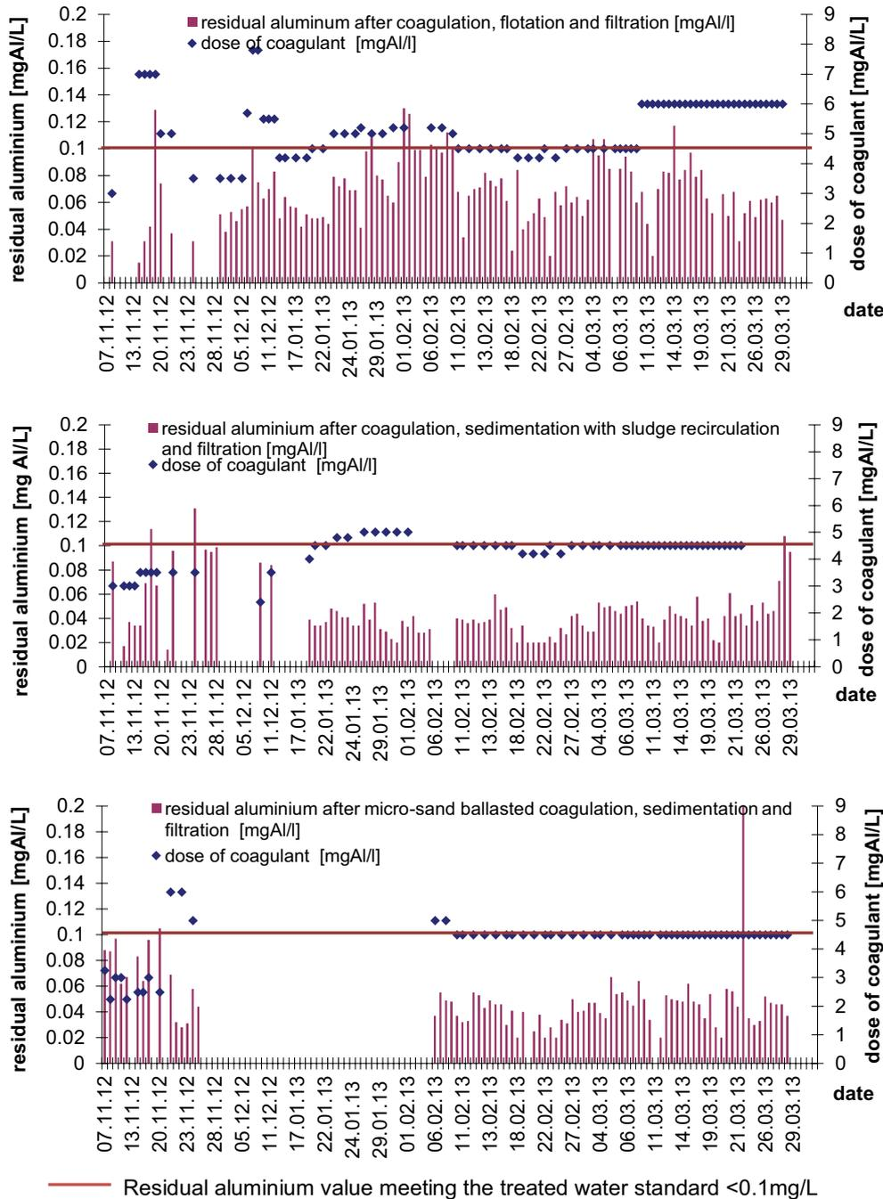
Fig. 6. Residual aluminum in water after coagulation, flotation or sedimentation and filtration depending on the coagulant dose.
