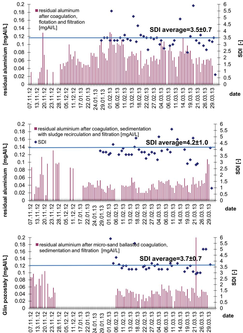
Fig. 8. Changes in SDI and residual aluminum in water after coagulation, sedimentation or flotation and filtration with an average SDI value.
