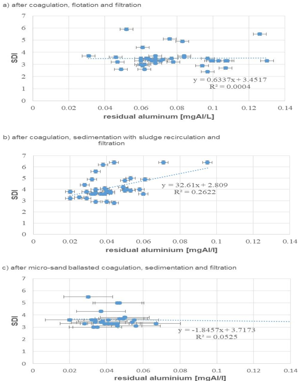
Fig. 9. Relationship between the concentration of the residual aluminum and the SDI in water after the coagulation, sedimentation or flotation, and filtration processes.
