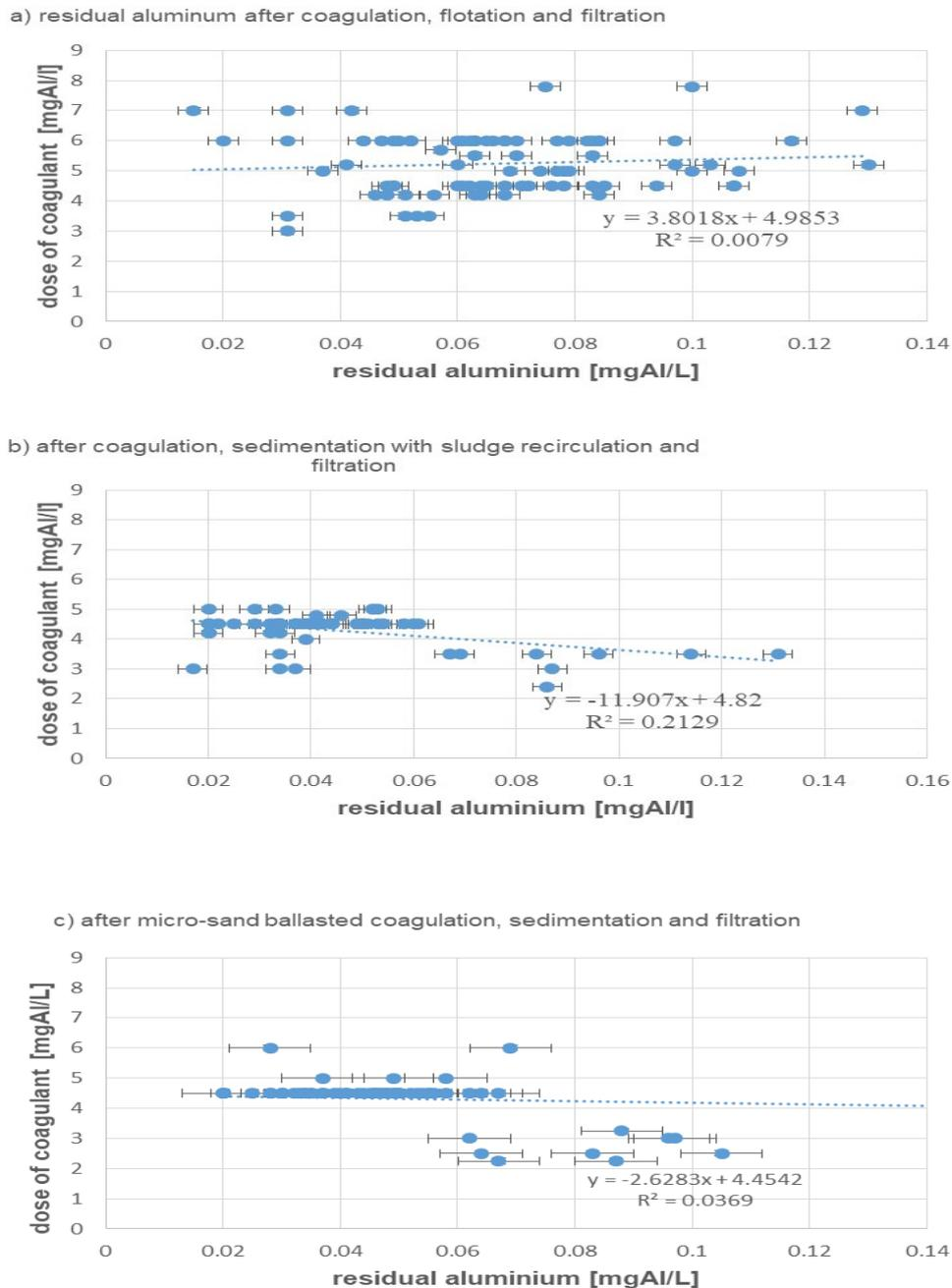
Fig. 7. Relationship between the concentration of the residual aluminum and the dose of coagulant in the water after the coagulation, flotation or sedimentation, and filtration processes.
