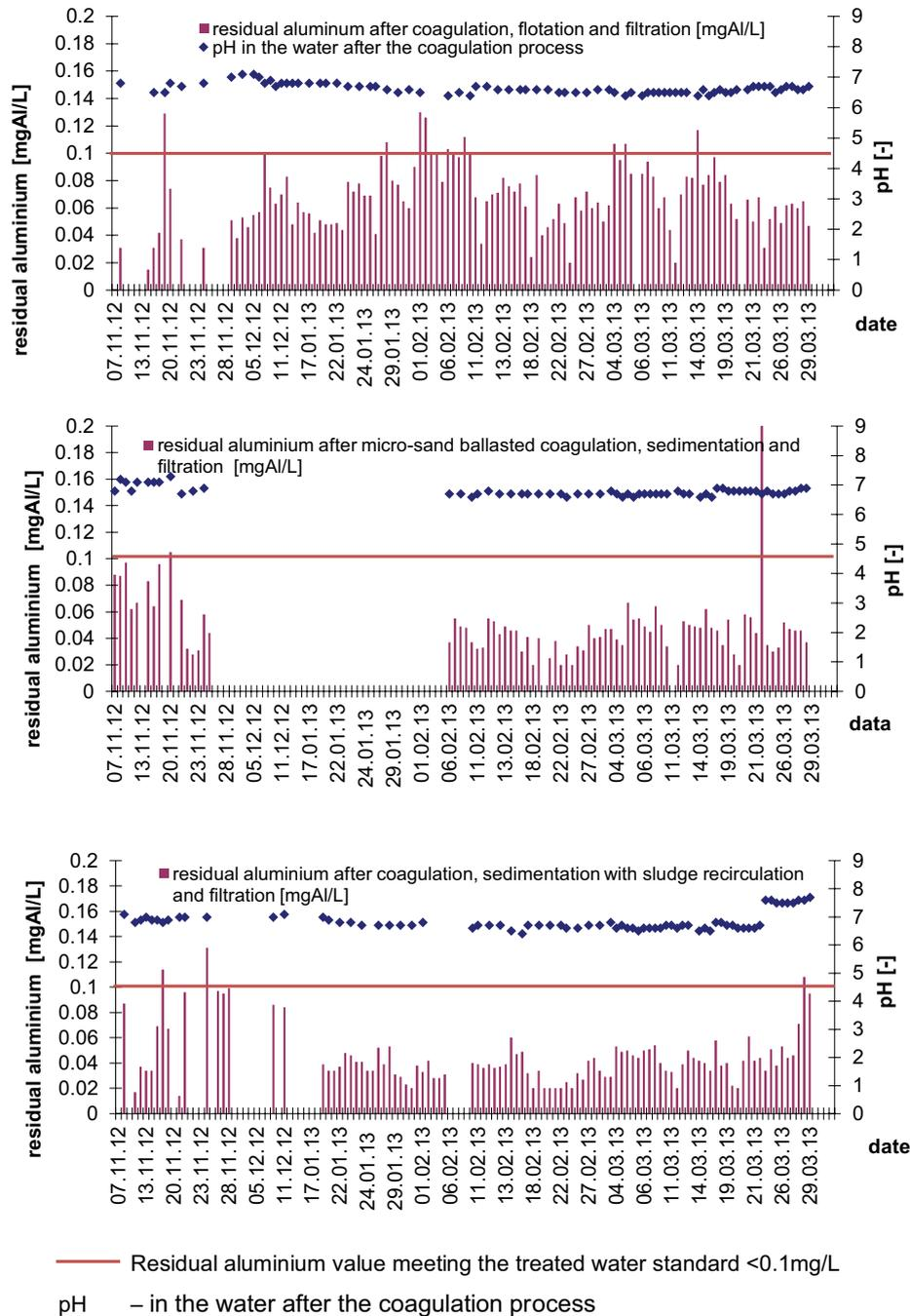
Fig. 4. Residual aluminum in water after coagulation, flotation or sedimentation and filtration depending on the pH.
