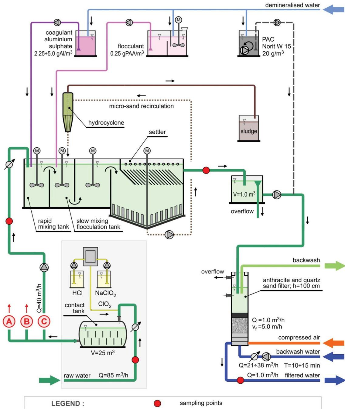
Fig. 3. Flow chart of the technological processes analyzed during the micro-sand ballasted coagulation with sedimentation and filtration.
