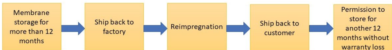
Fig. 1. Flow diagram of the present storage extension process.
