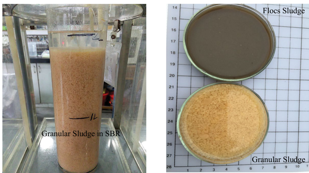
Fig. 1. Aerobic granular sludge from the lab-scale reactor and activated floc sludge from the secondary sedimentation tank.
