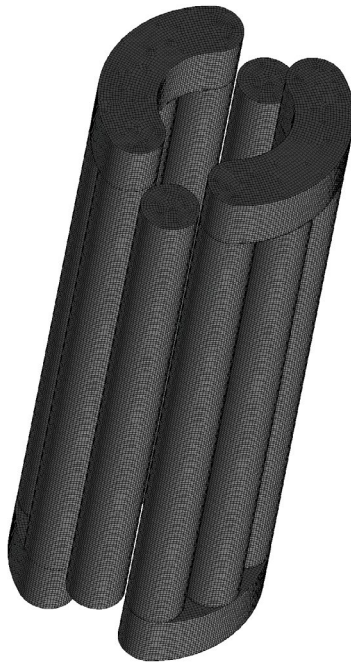
Fig. 3. Schematic diagram of model structure meshing parameters of the rotor.
