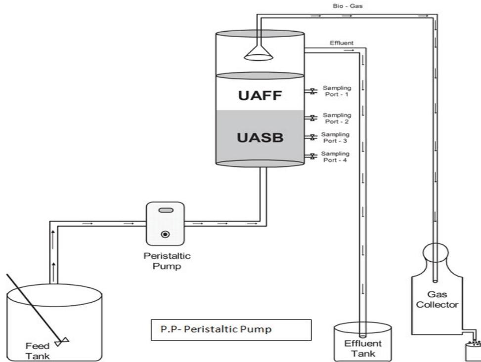
Fig. 1. Schematic diagram of the laboratory-scale experimental setup.
