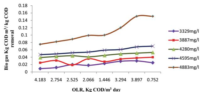
Fig. 4. Performance of OLR with respect to percentage COD removal efficiency.
