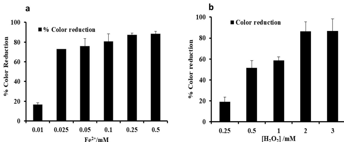
Fig. 6. The color reduction of STW with different Fenton conditions at pH = 3, temperature = 30°C: (a) with different  $\text{Fe}^{2+}$  dosages at 2.0 mM  $\text{H}_2\text{O}_2$  concentration and (b) with different of  $\text{H}_2\text{O}_2$  dosages at 0.5 mM  $\text{Fe}^{2+}$  concentration.
