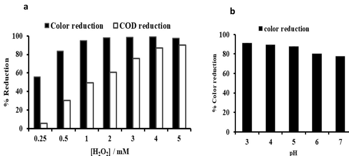
Fig. 4. (a) Variation of color and COD reduction at  $[\text{Fe}^{2+}]:[\text{H}_2\text{O}_2] = 1:10$  ratio and (b) pH dependence of color reduction at  $[\text{Fe}^{2+}]:[\text{H}_2\text{O}_2] = 1:10$  ratio.
