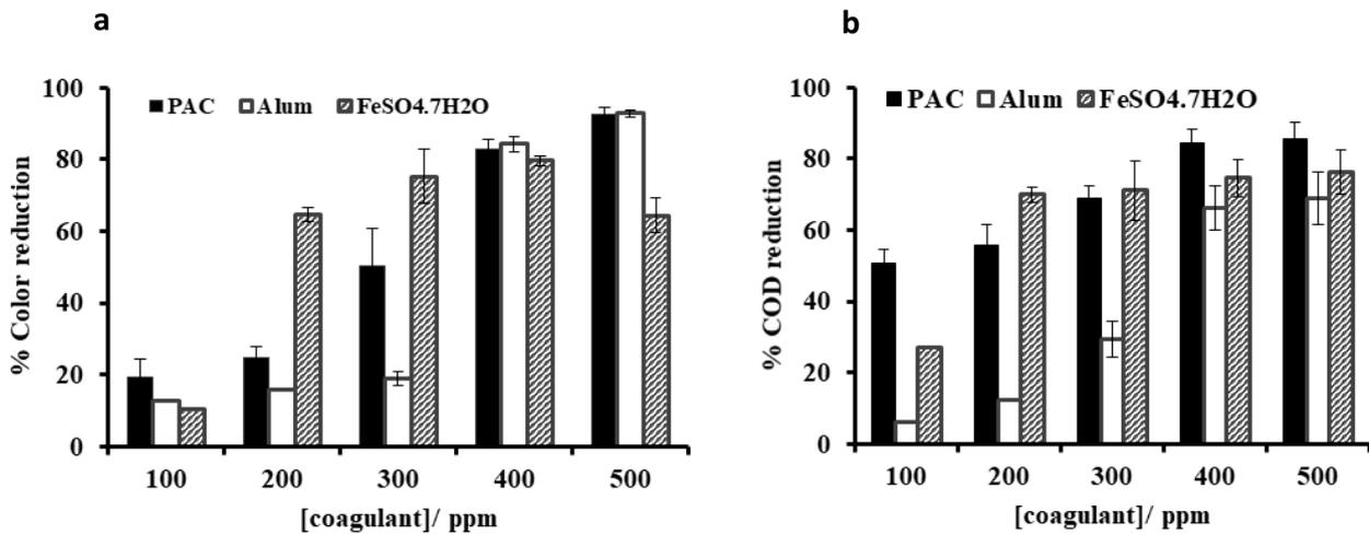
Fig. 7. (a) Color and (b) COD reduction of real textile wastewater by different coagulants at pH = 9, temperature = 30°C.
