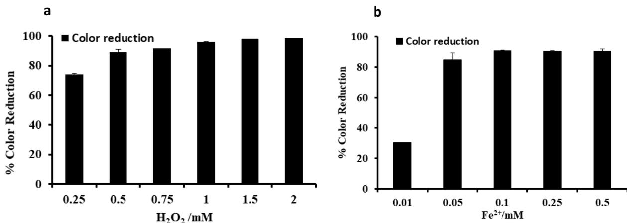
Fig. 8. Percentage color reduction of the real textile water (RTW) at different: (a) H<sub>2</sub>O<sub>2</sub> and (b) Fe<sup>2+</sup> concentrations at pH = 3, T = 30°C.
