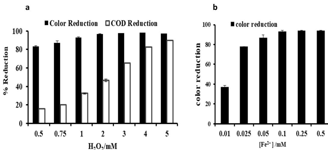
Fig. 3. Percentage color and COD reduction under different Fenton conditions: (a) variation with  $\text{H}_2\text{O}_2$  concentrations at  $[\text{Fe}^{2+}] = 0.5$  mM and (b) variation with  $\text{Fe}^{2+}$  concentrations at  $[\text{H}_2\text{O}_2] = 1.0$  mM.
