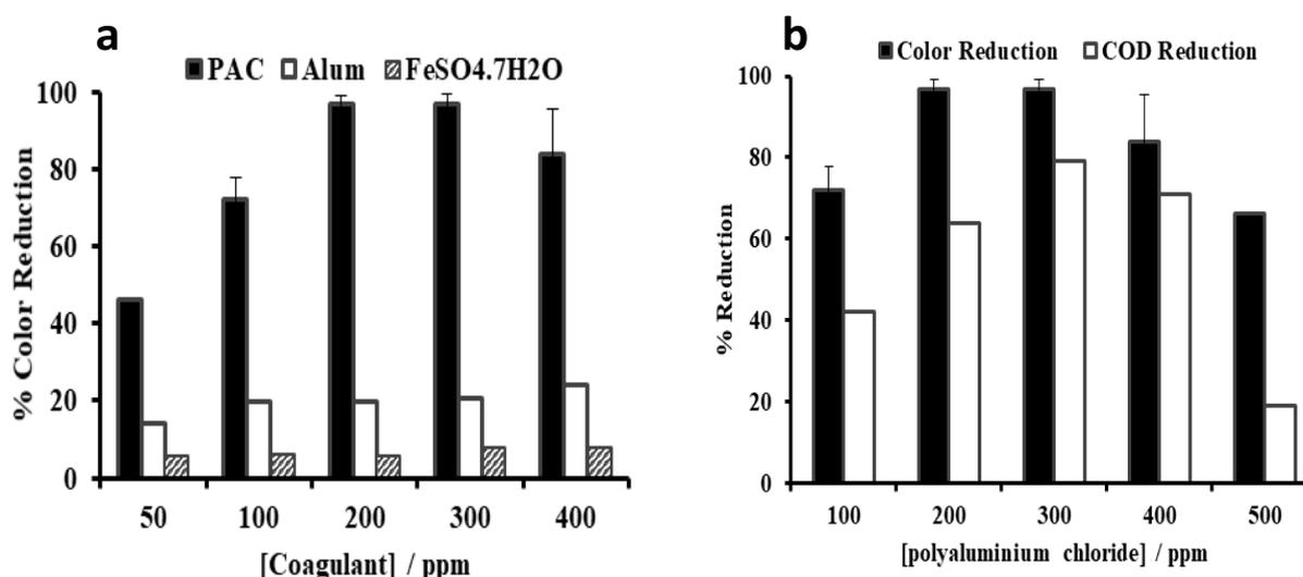
Fig. 2. (a) Color and (b) COD reduction of RB 5 with polyaluminium chloride at pH 9.
