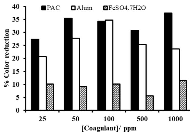
Fig. 5. The color reduction of 100 ppm STW with three different coagulants at pH = 9.
