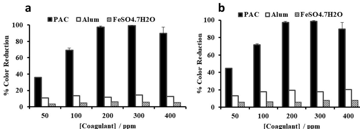
Fig. 1. Variations in the color reduction of 100 ppm RB 5 dye solution by three different coagulants with coagulant dosage and pH (a) pH 5 and (b) pH 7.
