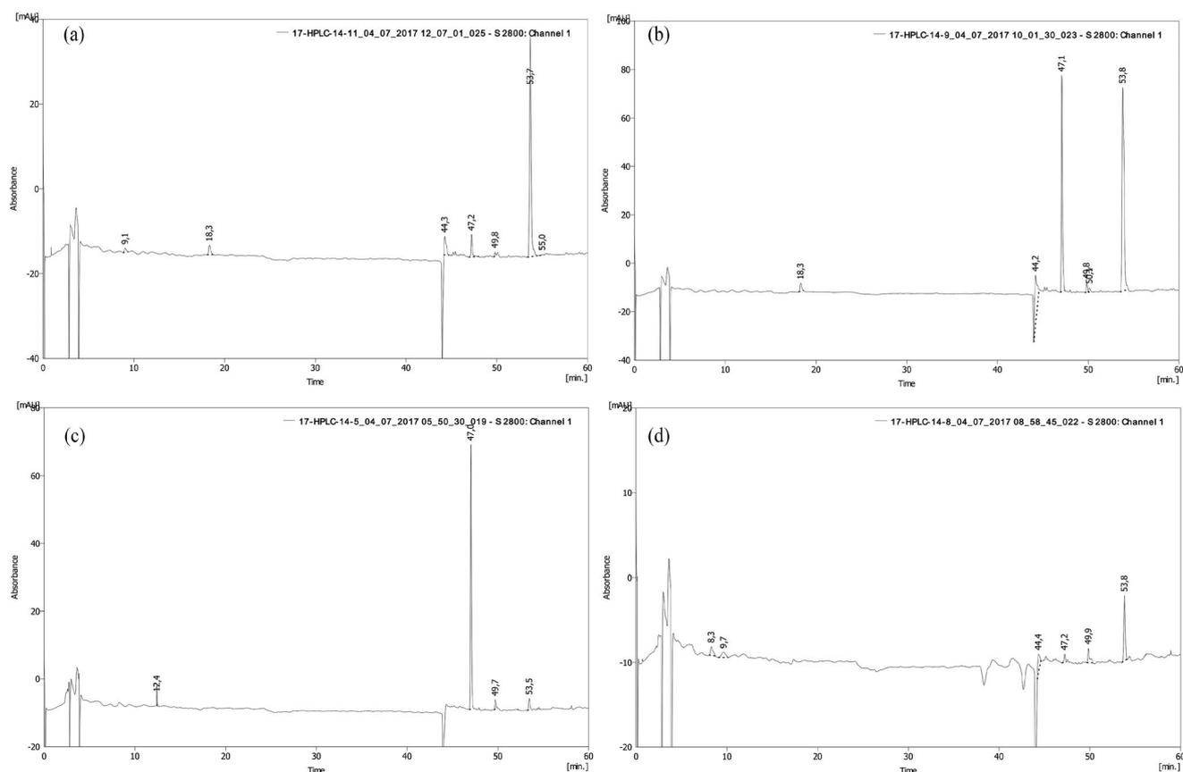
Fig. 9. High performance liquid chromatography chromatogram of phenolic compounds for (a) sand 0–10 cm, (b) sand 10–20 cm, (c) sand 20–30 cm, and (d) pozzolan.
