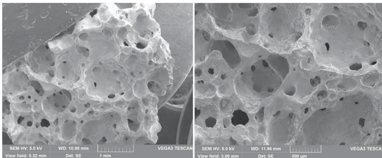
Fig. 2. Scanning electron microscopy (SEM) images of natural pozzolan at different zoom.
