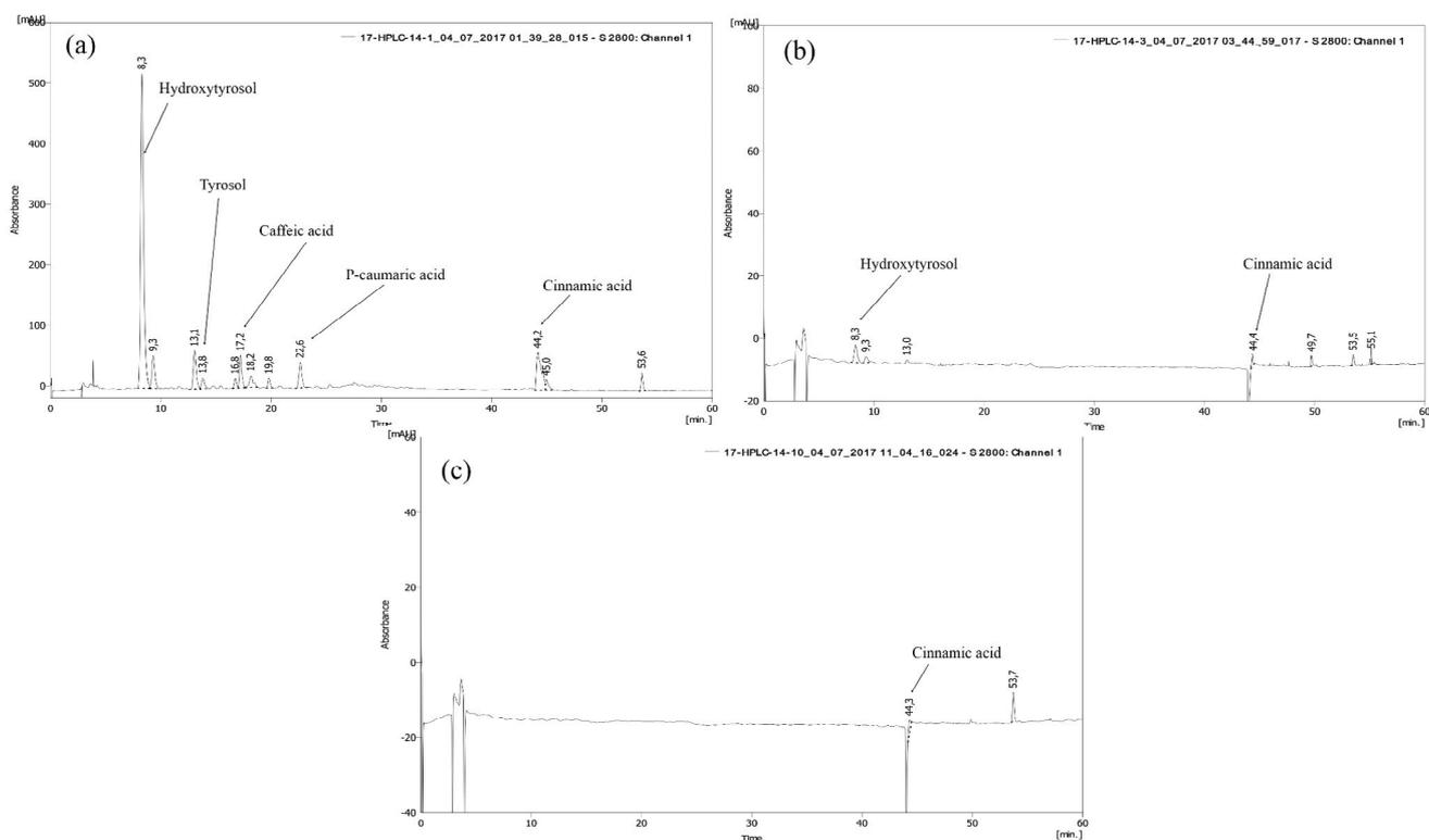
Fig. 8. High performance liquid chromatography chromatogram of phenolic compounds for (a) crude OMWW, (b) crude mixture OMWW + MWW, and (c) treated mixture.
