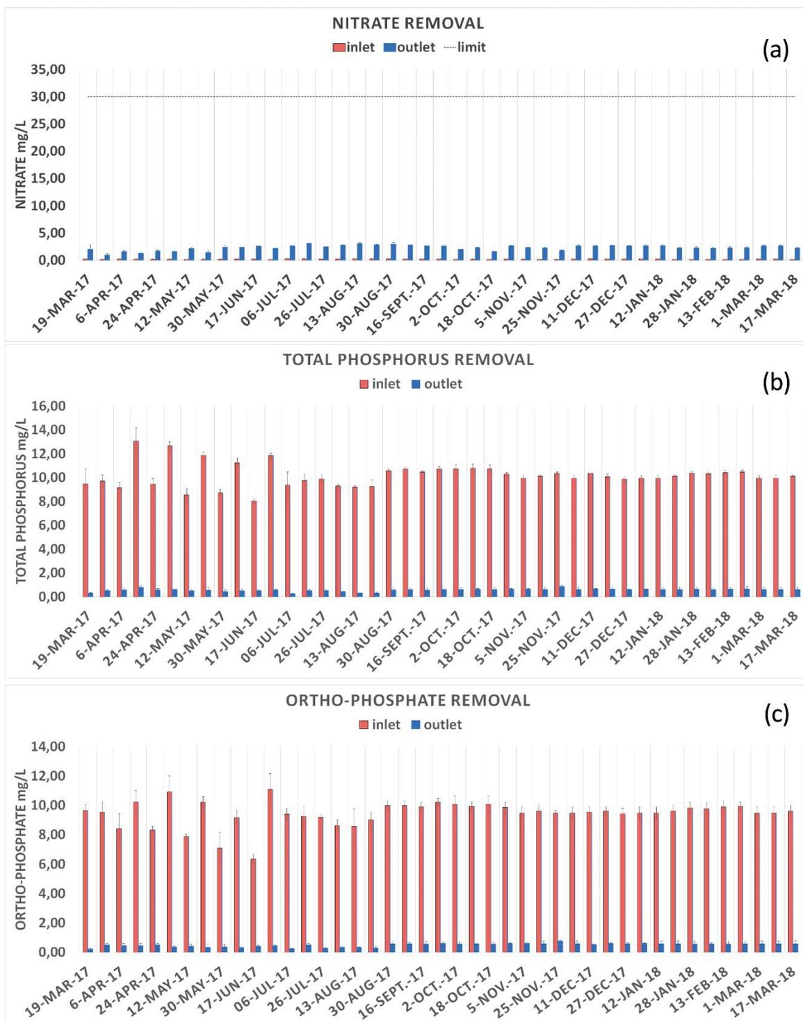
Fig. 5. Evolution of nitrate (a), phosphorus (b), and ortho-phosphate (c) during the treatment period.
