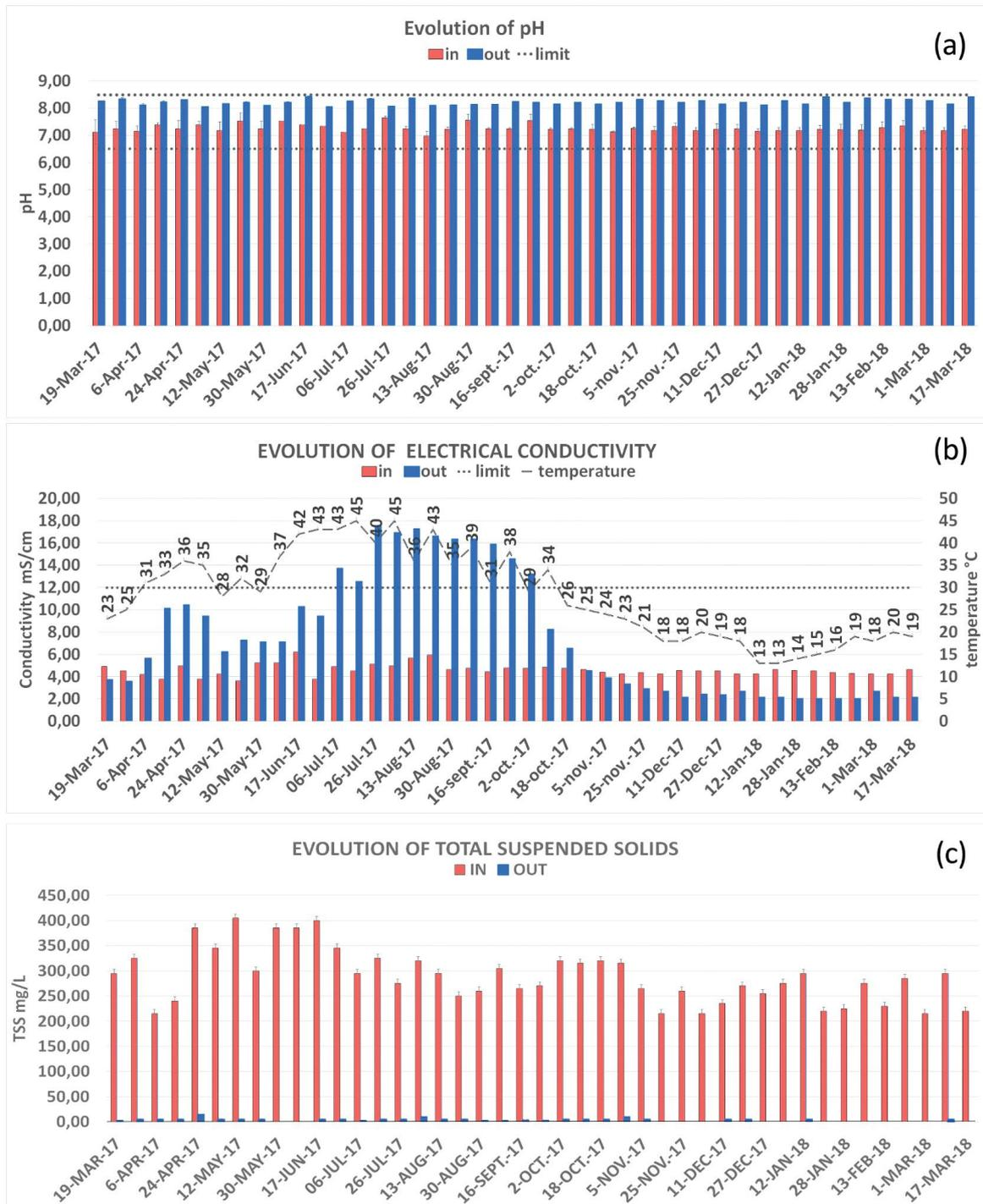
Fig. 3. Evolution of pH (a), electrical conductivity (b), and total suspended solids (c) during the treatment period.
