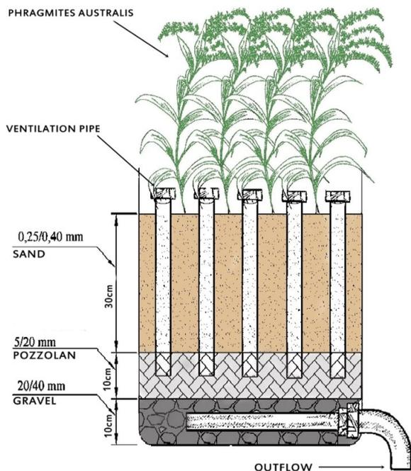
Fig. 1. Diagram of the pilot scale constructed wetland with vertical flow.
