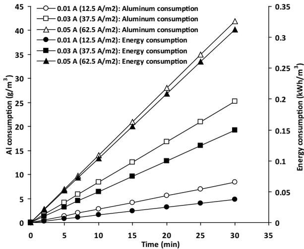
Fig. 5. Aluminum and energy consumption as a function of electrolysis time for different applied current densities.
