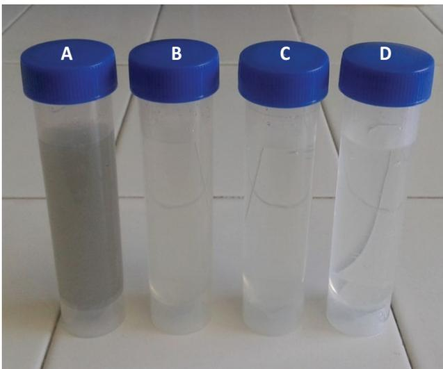
Fig. 8. Margarine effluent before (a) and after treatment by electrocoagulation [ $12.5 \text{ A/m}^2$  (b),  $37.5 \text{ A/m}^2$  (c) and  $62.5 \text{ A/m}^2$  (d)].
