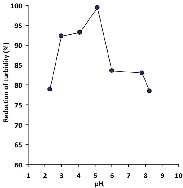
Fig. 2. Effect of pH on the treatment of margarine effluent by the electrocoagulation process.
