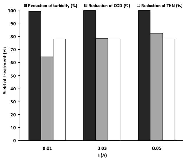
Fig. 7. Reduction of turbidity, COD and TKN of margarine effluent as a function of current intensity applied during an electrolysis period of 15 min.
