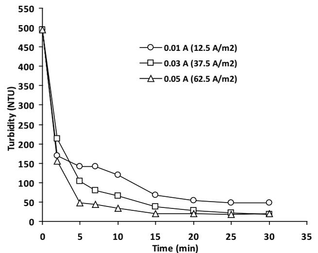
Fig. 4. Effect of electrolysis time on the turbidity of margarine effluent.
