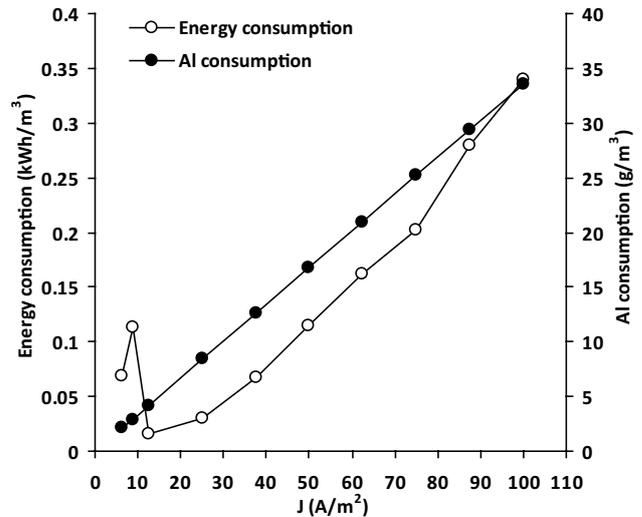
Fig. 6. Aluminum and energy consumption as a function of current density applied during an electrolysis period of 15 min.
