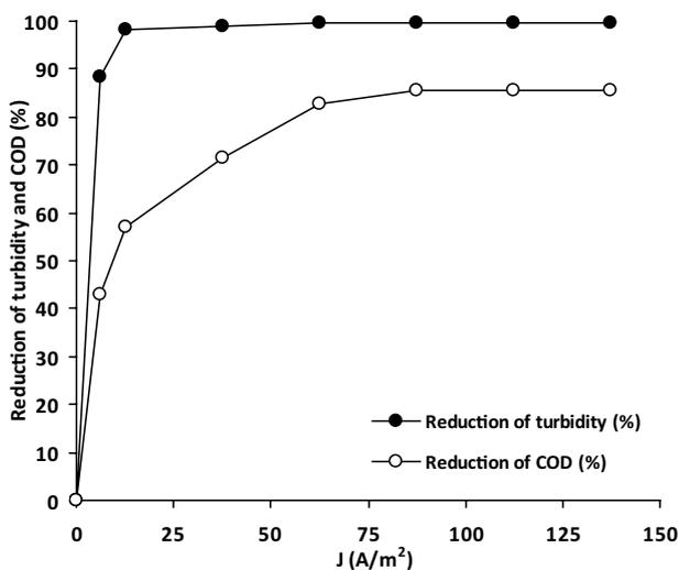
Fig. 3. Effect of current density on the reduction of turbidity and COD of margarine effluent.
