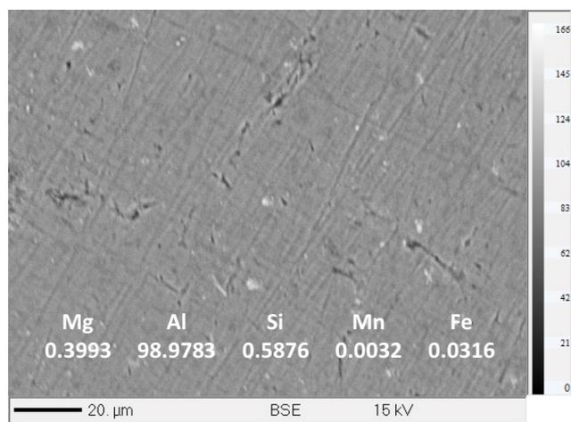
Fig. 1. Electron probe microanalysis of aluminum electrodes.
