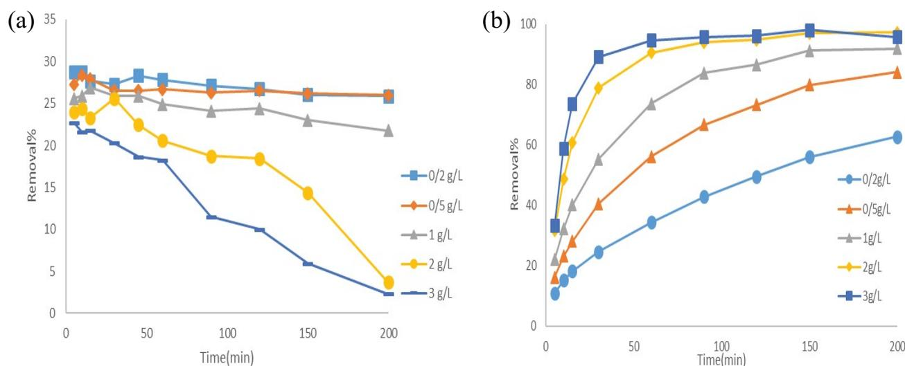
Fig. 8. Effect of adsorbent dosage in the efficiency of metronidazole removal by magnetic PAC (a) and magnetic GAC (b) [metronidazole concentration = 20 mg/L, pH (magnetic PAC) = 3, pH (magnetic GAC) = 7, and  $v = 300$  rpm].
