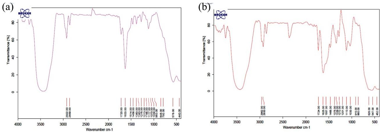
Fig. 1. FT-IR spectrum of magnetic PAC (a) and magnetic GAC (b).
