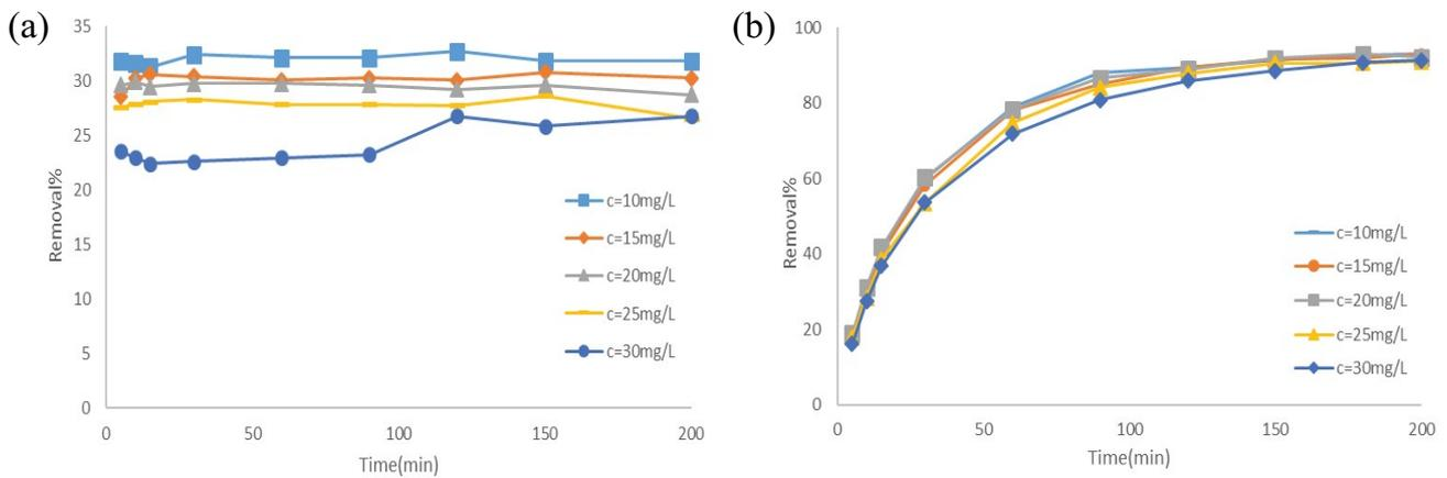
Fig. 9. Effect of the contact time and initial metronidazole concentration in the efficiency of metronidazole adsorption by magnetic PAC (a) and magnetic GAC (b) [pH (magnetic PAC) = 3, dose (magnetic PAC) = 0/2 g/L, pH (magnetic GAC) = 7, dose (magnetic GAC) = 1 g/L, and  $v = 300$  rpm].
