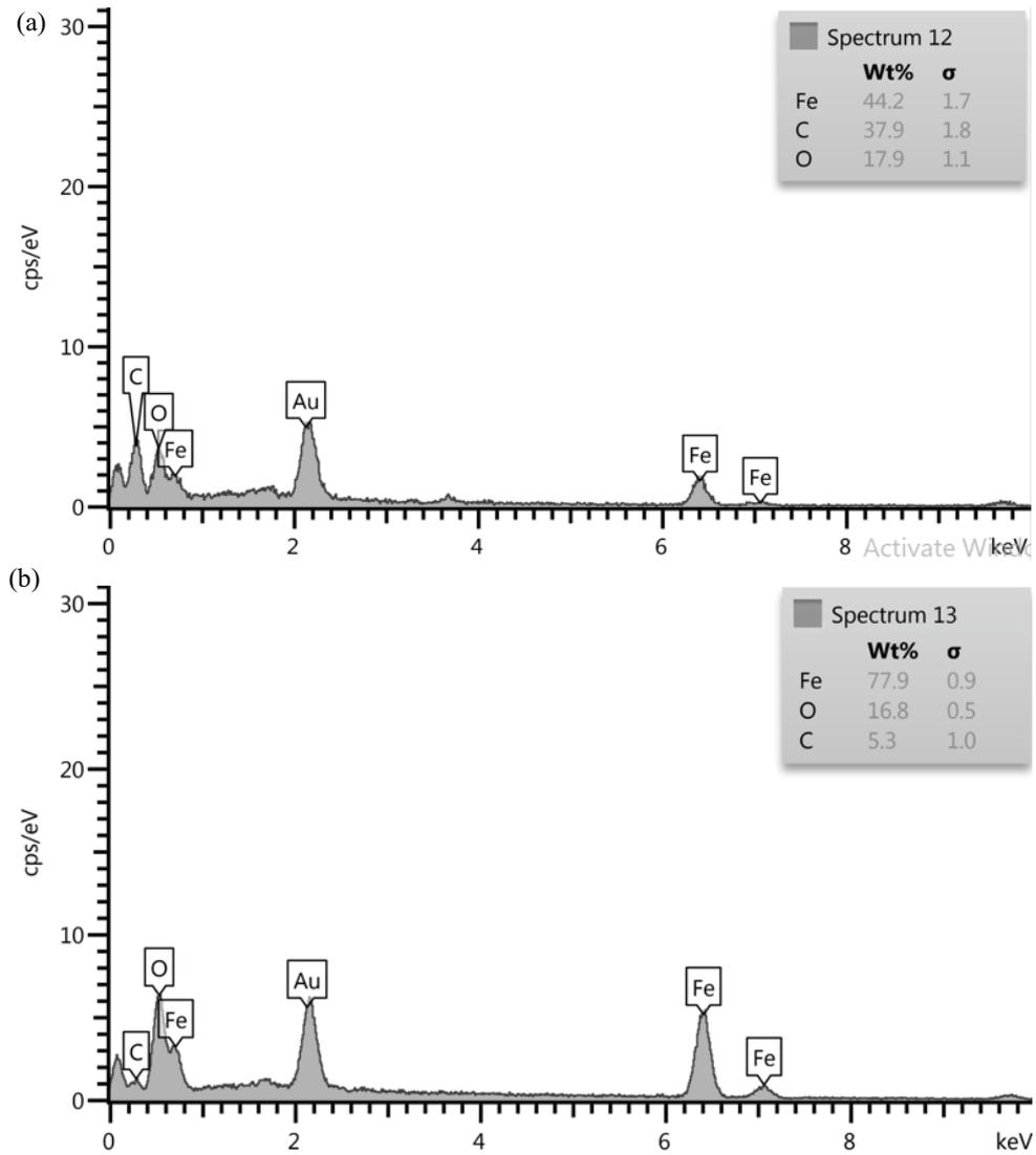
Fig. 6. EDS analysis of magnetic PAC (a) and magnetic GAC (b).
