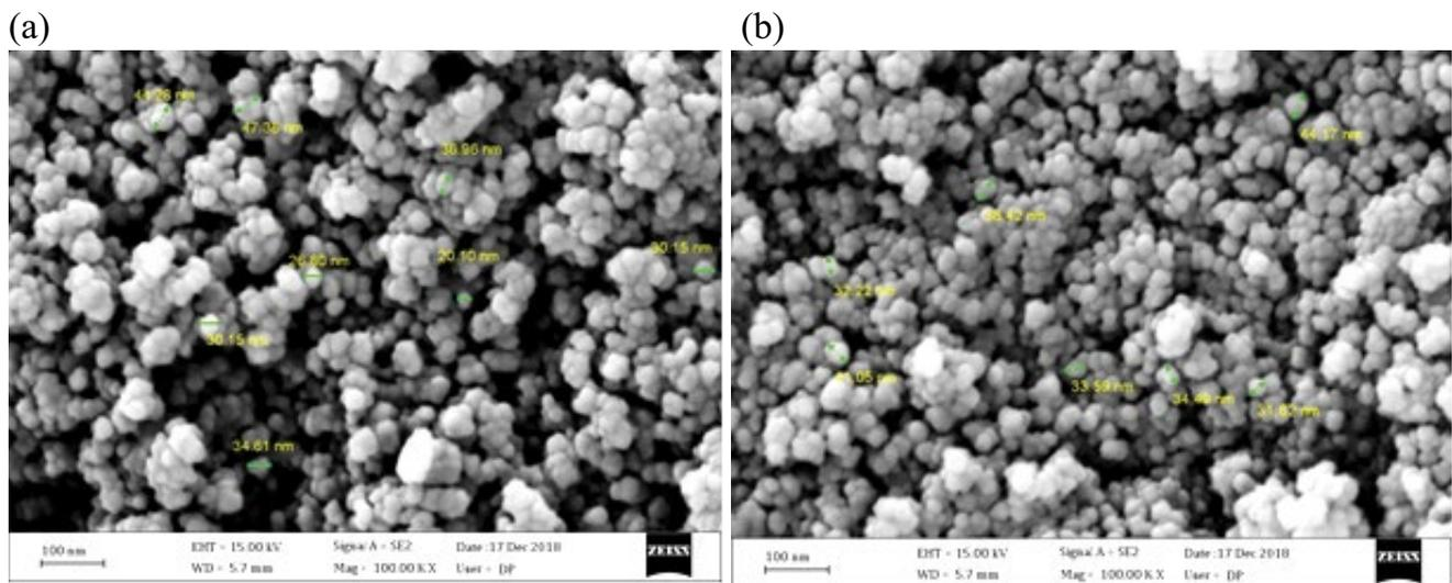
Fig. 4. SEM image of magnetic PAC (a) and magnetic GAC (b).
