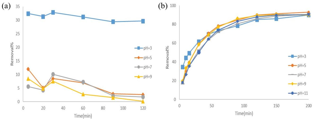
Fig. 7. Effect of changes in pH values in the efficiency of metronidazole removal by magnetic PAC (a) and magnetic GAC (b) [metronidazole concentration = 20 mg/L, adsorbent dosage = 1 g/L, and  $v = 300$  rpm].
