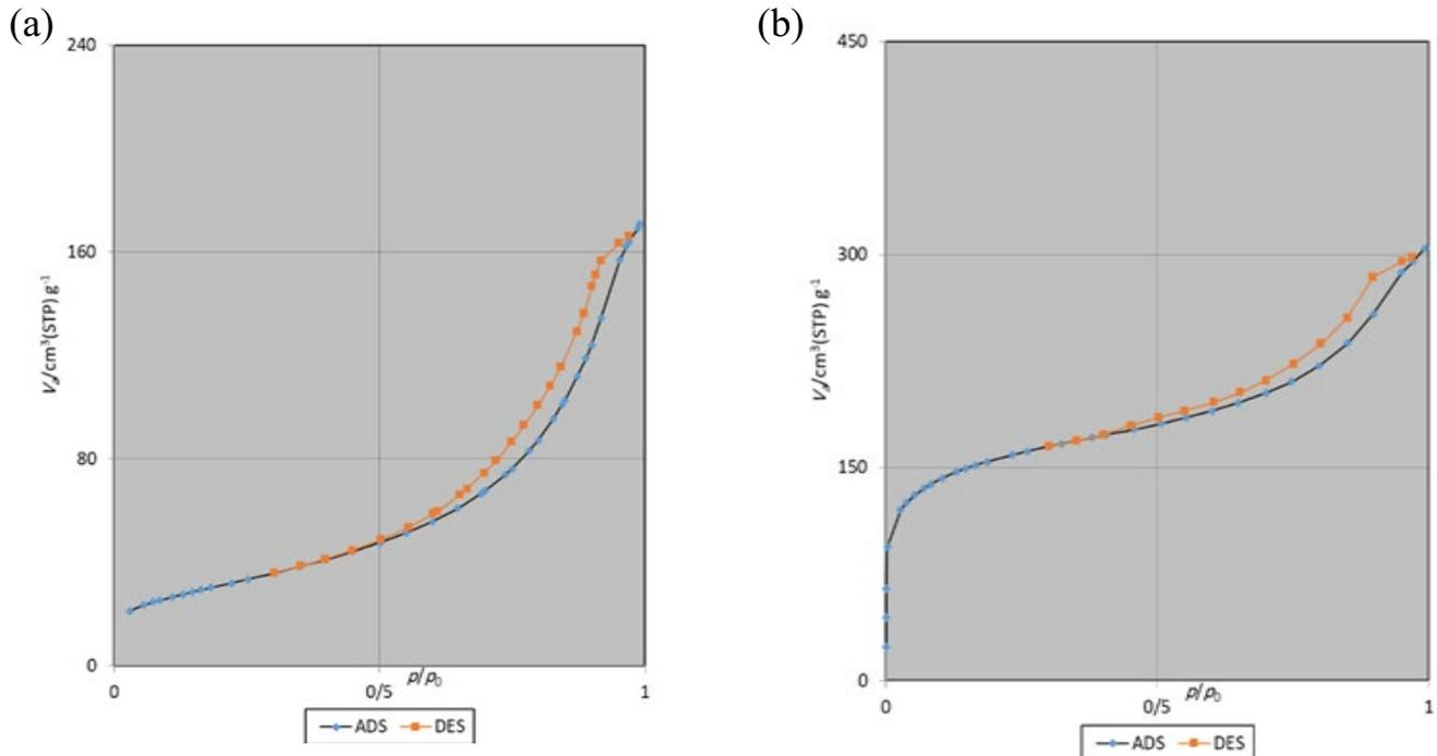
Fig. 5. Adsorption and desorption hysteresis of magnetic PAC (a) and magnetic GAC (b).
