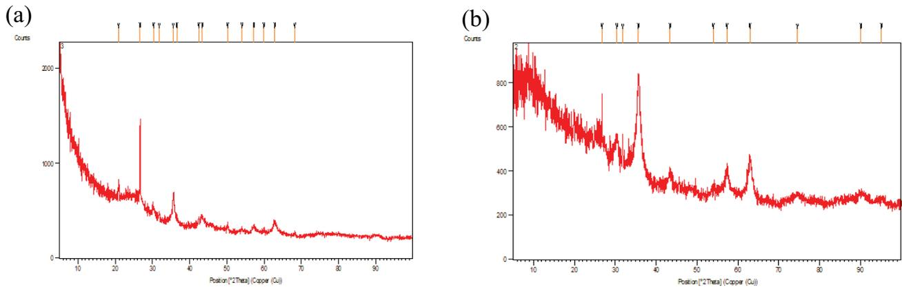
Fig. 3. XRD spectrum of magnetic PAC (a) and magnetic GAC (b).
