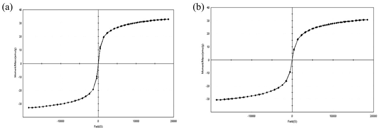
Fig. 2. VSM curve of magnetic PAC (a) and magnetic GAC (b).
