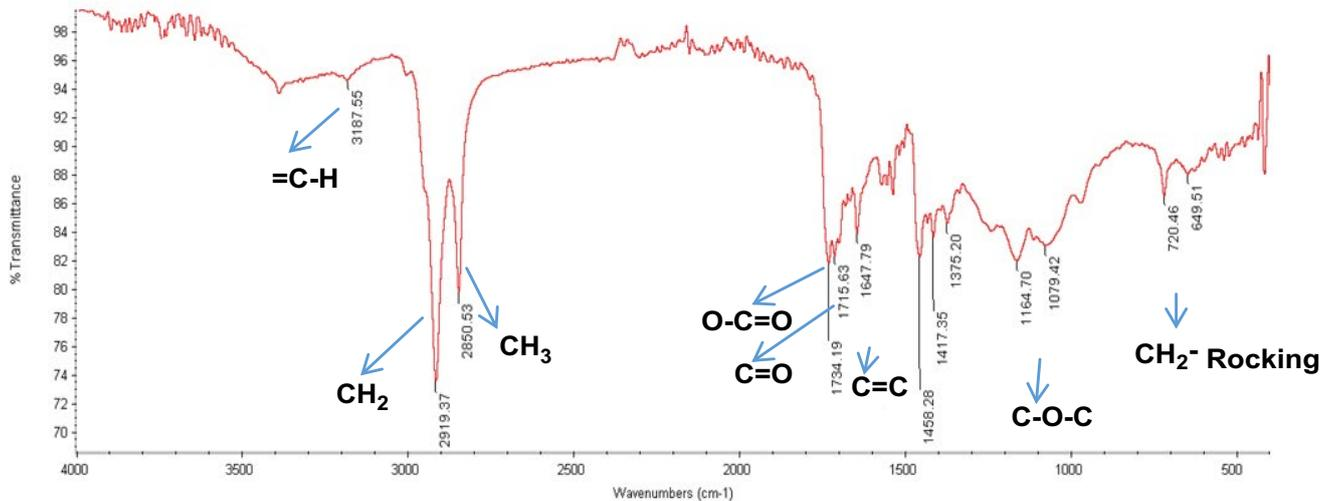
Fig. 8. FTIR spectrum of chemical constituents extracted from *S. filipendula*.
