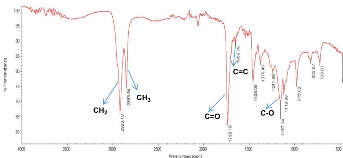
Fig. 5. FTIR spectrum of fatty acids methyl esters extracted from *S. denticulatum*.
