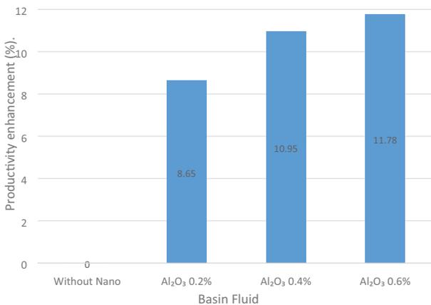
Fig. 13. Percent increase in the distilled water production for the pyramid solar still at  $Al_2O_3$  nanoparticles concentrations.
