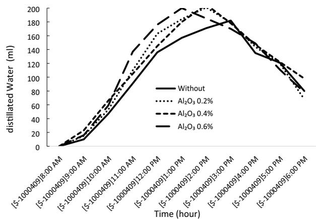
Fig. 7. Variation of distilled water production for pyramid solar still with and without different concentrations of Al<sub>2</sub>O<sub>3</sub> nanoparticles.
