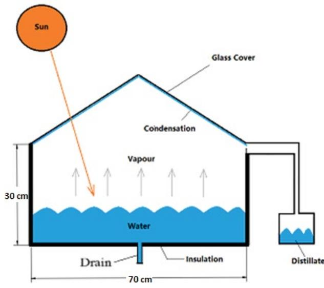
Fig. 1. Schematic of the system.
