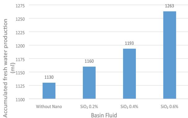
Fig. 8. Total amount of freshwater for solar still with and without utilizing different concentrations of silica oxide  $SiO_2$ .
