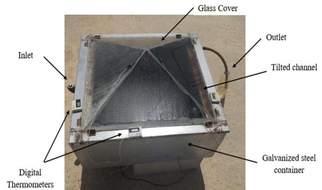
Fig. 3. pyramid solar still that used in the experiment.
