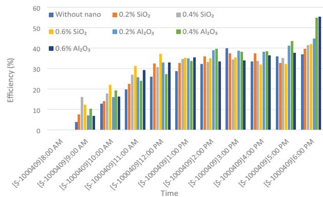
Fig. 14. Hourly variation of the pyramid solar still efficiency during experimental days.
