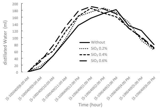
Fig. 6. Variation of distilled water production for pyramid solar still with and without different concentrations of SiO<sub>2</sub> nanoparticles.
