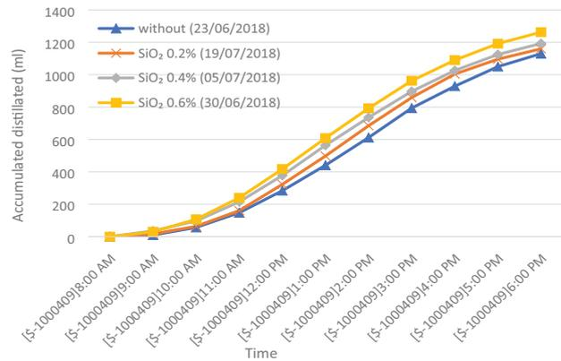
Fig. 9. Accumulative amounts of freshwater produced from solar still with and without utilizing different concentration of silica oxide  $SiO_2$ .
