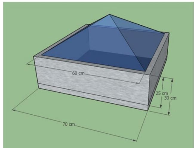
Fig. 2. 3D Model for pyramid solar still.
