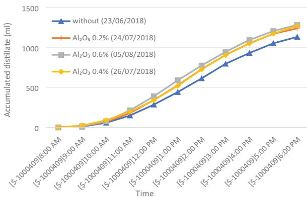
Fig. 12. Accumulative amounts of freshwater produced from solar still with and without utilizing different concentrations of aluminum oxide  $Al_2O_3$ .
