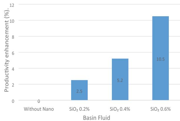
Fig. 10. Percent increase in the distilled water production for the pyramid solar still at  $SiO_2$  nanoparticles concentrations.
