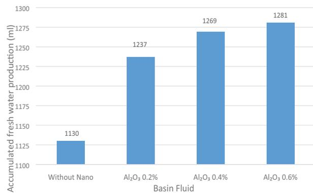
Fig. 11. Total amount of freshwater for solar still with and without utilizing different concentration of aluminum oxide  $Al_2O_3$ .
