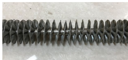
Fig. 7. (a) Schematic illustration of the experimental set-up for a single-cell, (b) three-dimensional CAD model of the experimental set-up, (c) bubble-column condenser, and (d) helical-fin heat exchanger (hot water flows through the inner pipe, and moist air flows outside).
