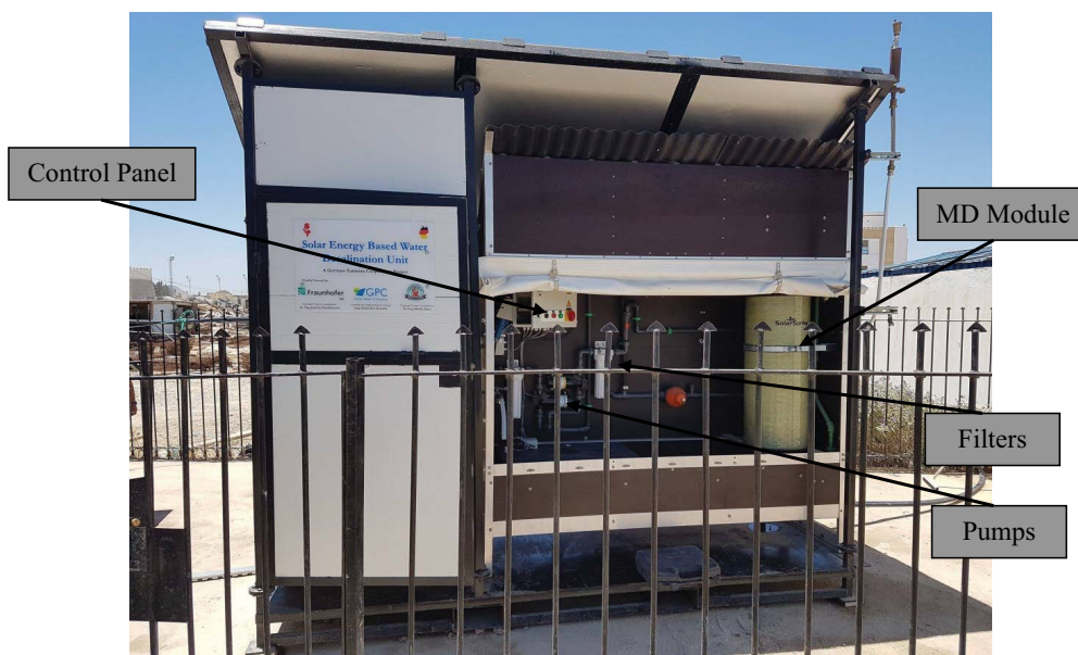
Fig. 4. Rear view of the solar membrane distillation pilot system.
