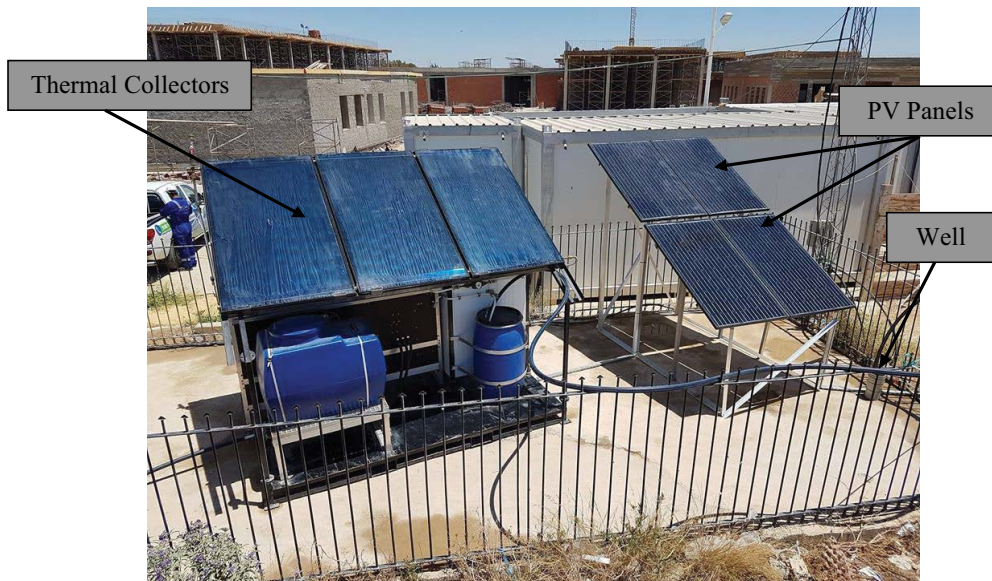
Fig. 3. Front view of the solar-membrane distillation pilot system.
