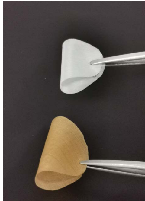
Fig. 15. Optical photographs show the robust flexibility of pristine and modified nylon mesh.
