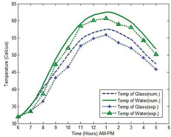
Fig. 10. Numerical and experimental measurements of the cover glass and basin water temperatures for 3 cm water depth and a cover slope angle 35° for summer.
