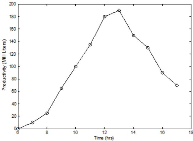
Fig. 8. Hourly rate of distilled water production in the solar still during a typical day of winter.
