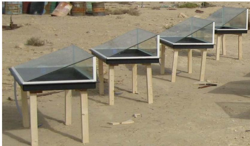
Fig. 1. Four sets of solar stills for experimental measurements. The slopes of glass covers are 25°, 30°, 35°, and 40° respectively.
