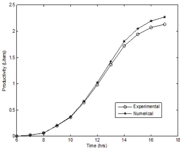
Fig. 14. Experimental and numerical comparison of productivity for 3 cm water depth and a cover slope angle 35° for summer.
