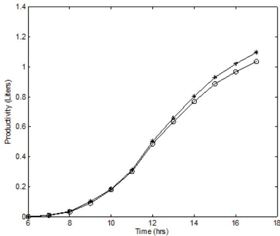
Fig. 16. Experimental and numerical comparison of productivity for 3 cm water depth and a cover slope angle 35° for winter.
