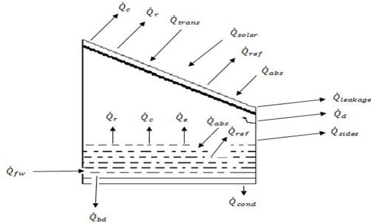
Fig. 2. Various heat transfer mechanisms taking place in a solar still.
