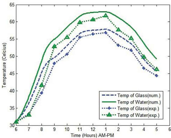
Fig. 9. Numerical and experimental measurements of the cover glass and basin water temperatures for 1 cm water depth and a cover slope angle 35° for summer.
