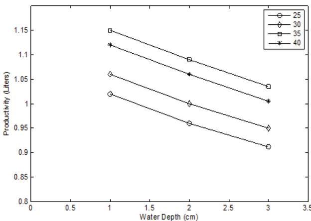
Fig. 6. Distilled water production of the solar still with varying water depths and four different cases of glass cover angles during a typical day of winter.
