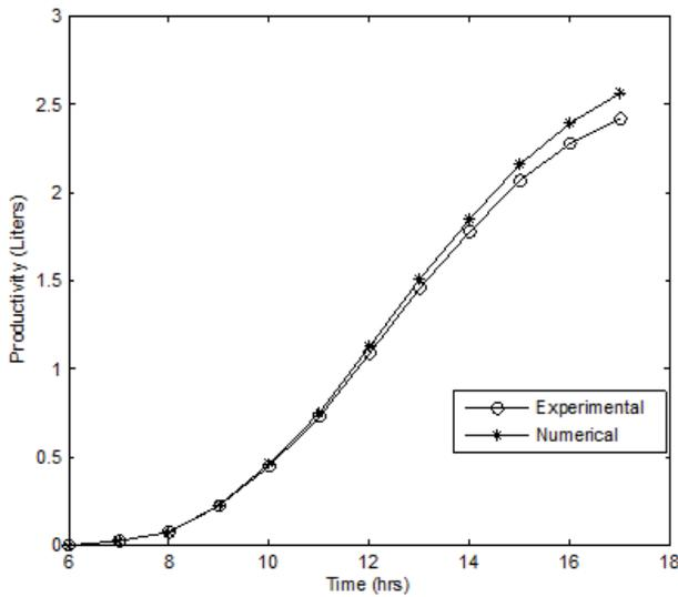
Fig. 13. Experimental and numerical comparison of productivity for 1 cm water depth and a cover slope angle 35° for summer.
