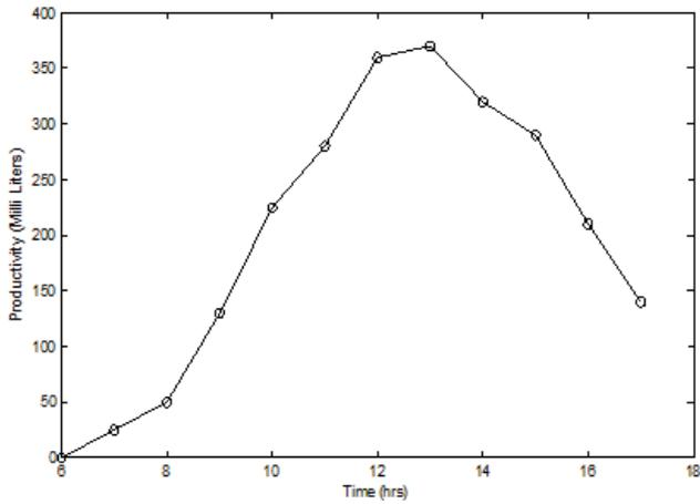
Fig. 7. Hourly rate of distilled water production in the solar still during a typical day of summer.
