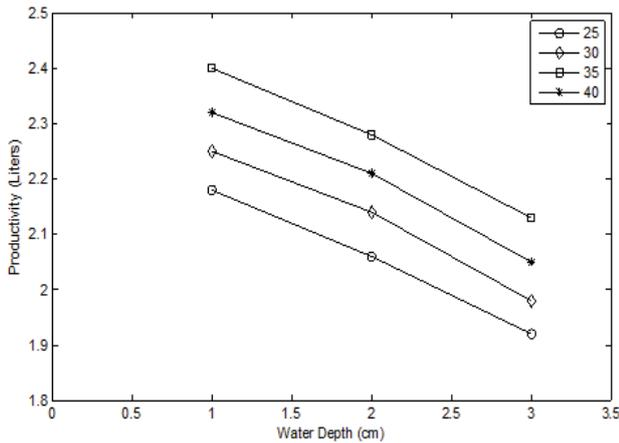
Fig. 5. Distilled water production of the solar still with varying water depths and four different cases of glass cover angles during a typical day of summer.
