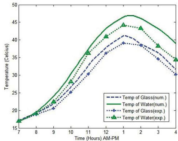
Fig. 12. Numerical and experimental measurements of the cover glass and basin water temperatures for 3 cm water depth and a cover slope angle 35° for winter.
