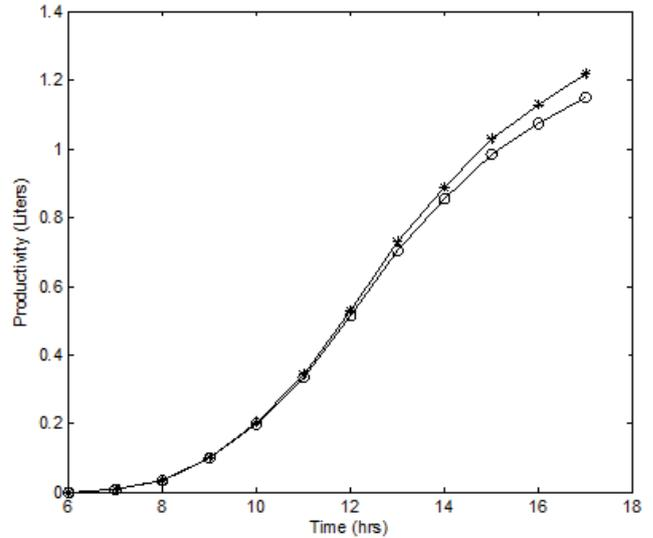
Fig. 15. Experimental and numerical comparison of productivity for 1 cm water depth and a cover slope angle 35° for winter.
