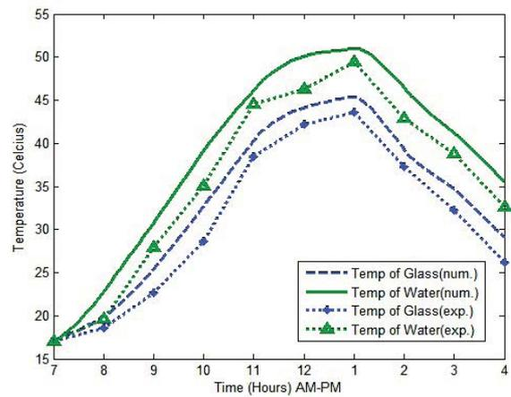
Fig. 11. Numerical and experimental measurements of the cover glass and basin water temperatures for 1 cm water depth and a cover slope angle 35° for winter.
