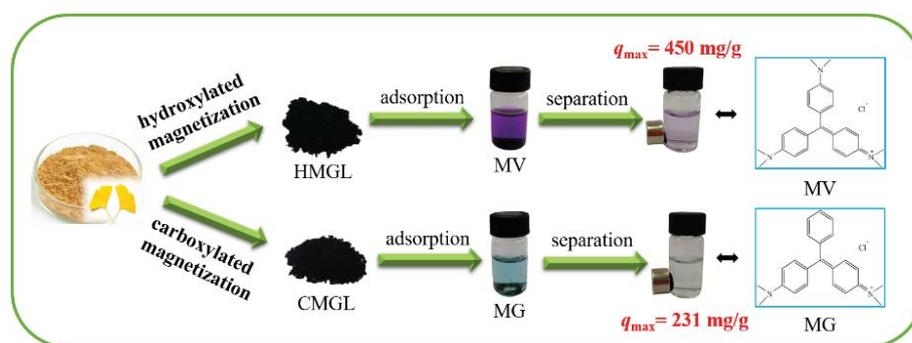
Fig. 1. Schematic illustration of the adsorption process.
