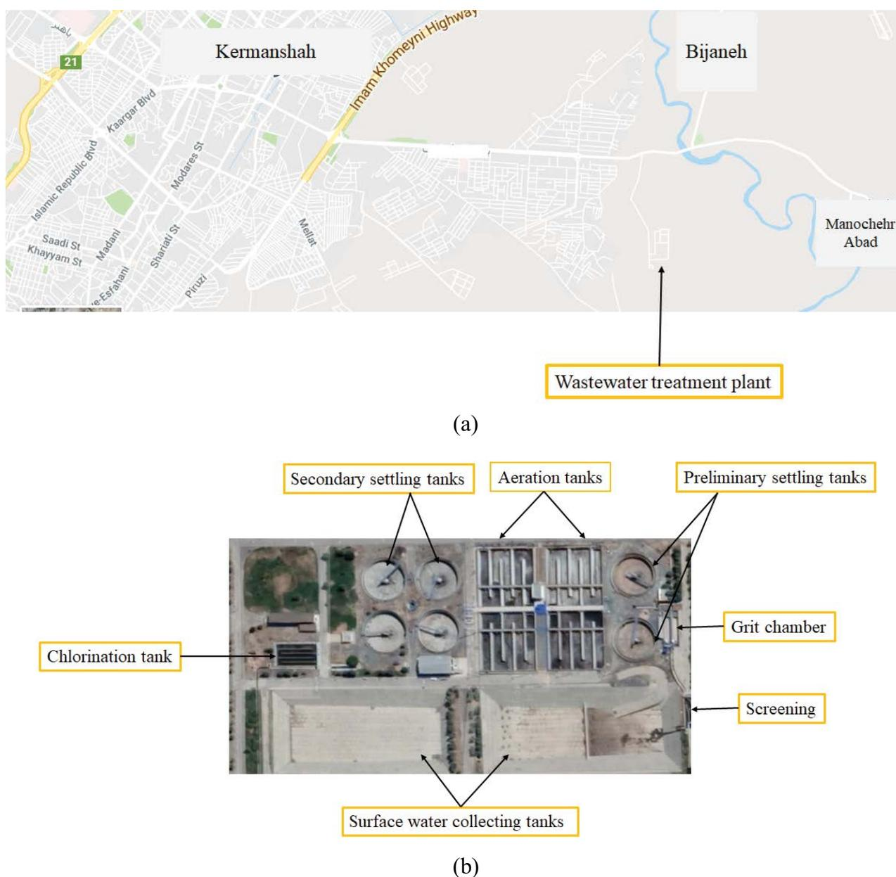
Fig. 1. (a) Geographical location and (b) process flow diagram of the Kermanshah's WWTP.
