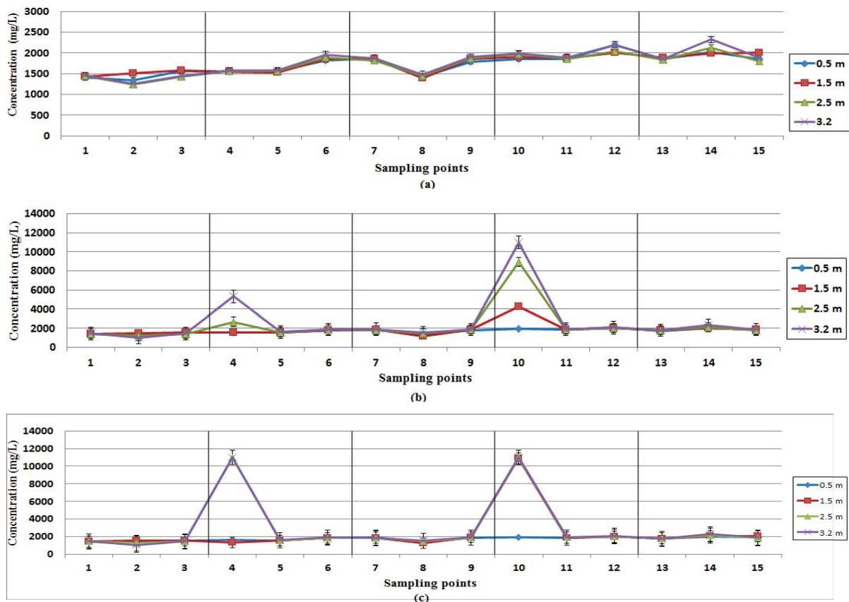
Fig. 10. Variations of the MLSS concentration at different depths of and different regions of the aeration tank (a) right, (b) middle, and (c) left sides.
