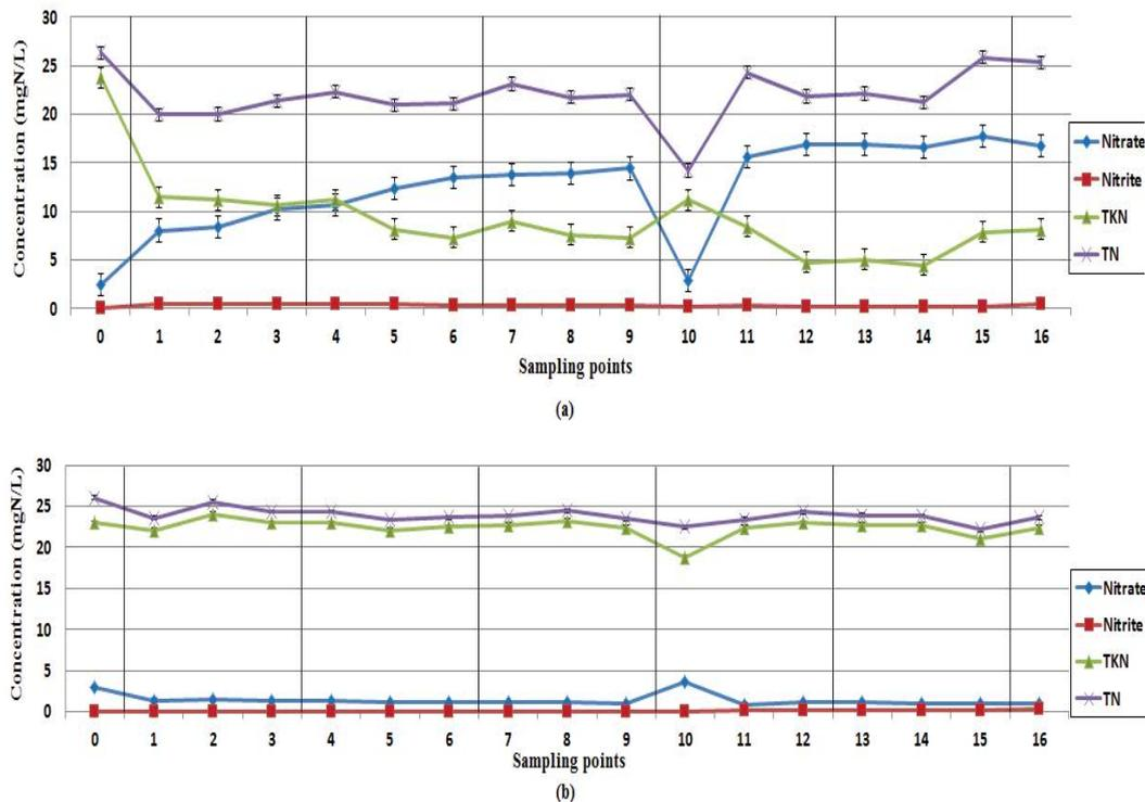
Fig. 9. Average variations of the nitrogenous compounds at the length of the aeration tank and different angles of (a) 30° and (b) 45°.
