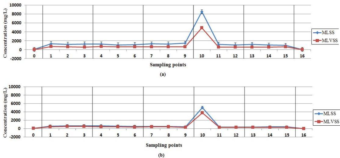
Fig. 4. Variations of the MLSS concentration at the length of the aeration tank at two different angles of aerators installation (a) 30° and (b) 45°.
