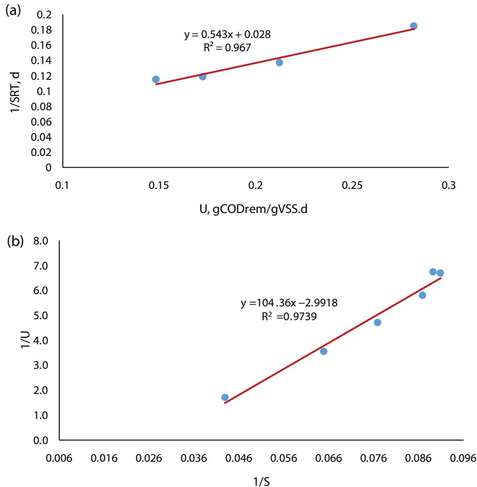
Fig. 11. Determination of the kinetic coefficients based on (a) specific microbial growth rate ( $U$ ) vs.  $1/SRT$  and (b) reverse COD removal ( $1/S$ ) vs. reverse specific microbial growth rate ( $1/U$ ).
