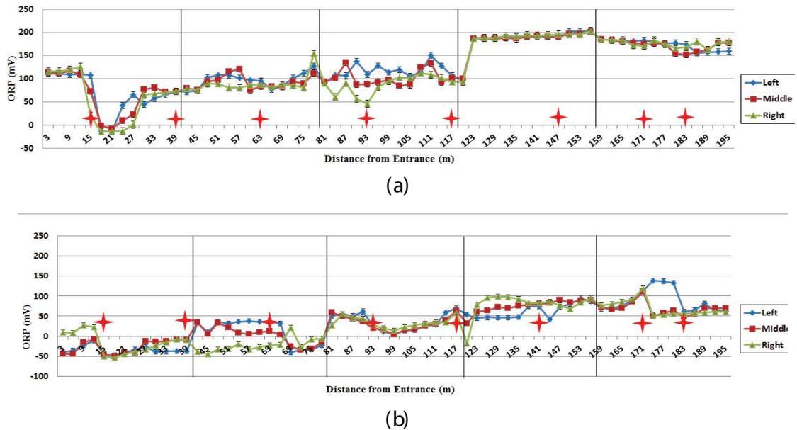
Fig. 6. Variations of ORP at the length of the aeration tank at the 0.5 m depth and the angles of (a) 30° and (b) 45°.
