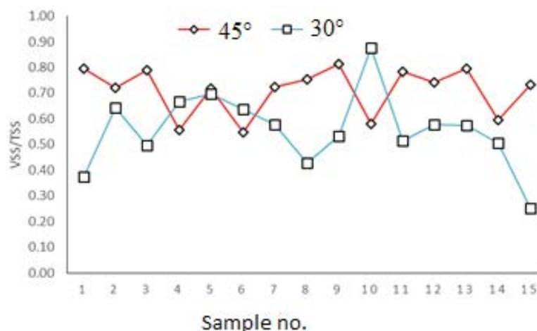
Fig. 12. Variations of the VSS to TSS ratio at the length of the aeration tank at different angles of the aerators installation.
