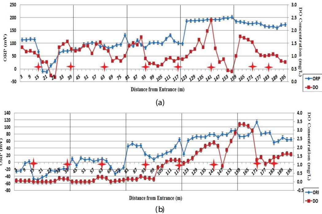
Fig. 7. Average variations of the DO and ORP at the length of the aeration tank and the 0.5 m depth, (a) at the 30° and (b) 45° angle.
