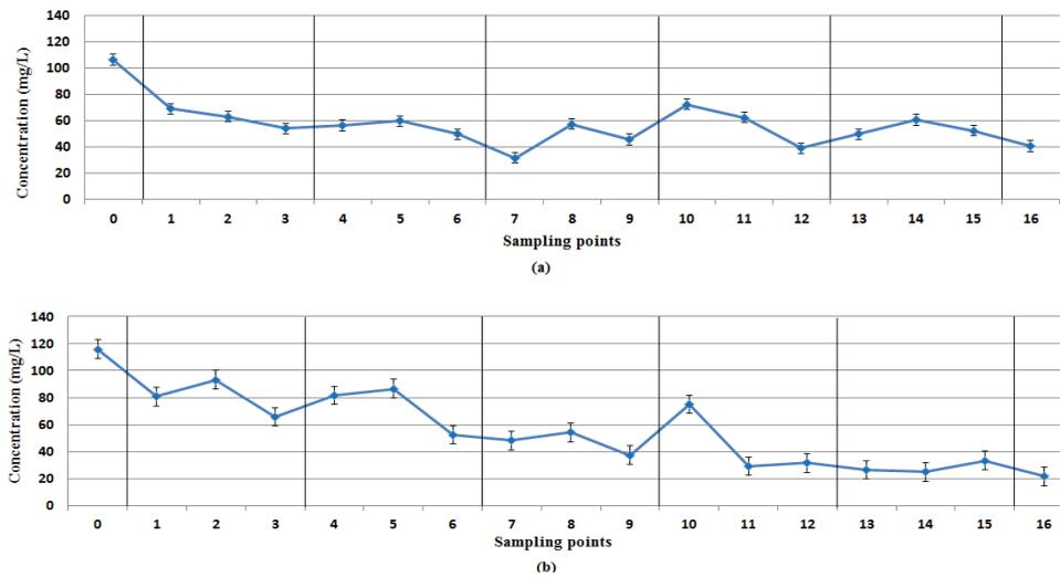
Fig. 8. Average variations of the COD concentration at the length of the aeration tank at angles of (a) 30° and (b) 45°.
