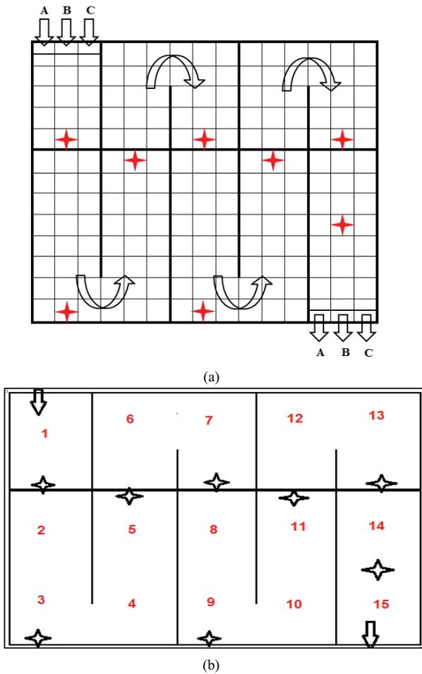
Fig. 3. Sampling regions for the measure of (a) DO and ORP, a sign of shows the aerator and (b) COD, BOD, MLSS, TN, and TP. Note: all aerators but last one were installed at the opposite direction of the flow.
