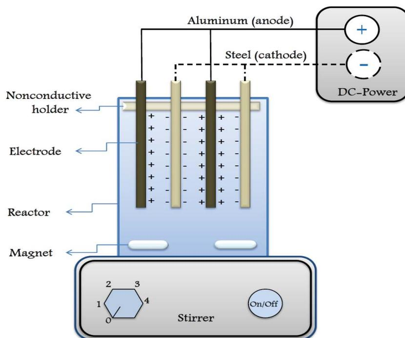
Fig. 1. Schematic diagram of the pilot reactor with cathodes and anodes parallel connections at monopolar electrodes.
