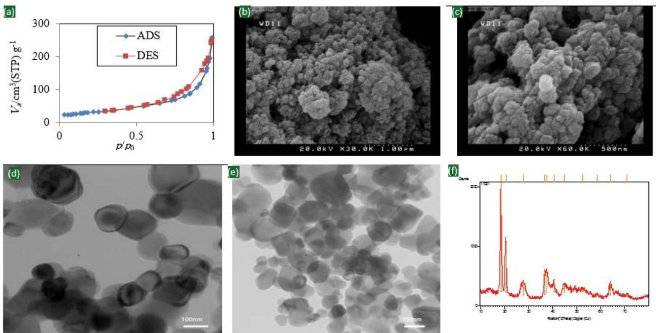
Fig. 6. BET plots of nitrogen adsorption–desorption isotherms (a), FE-SEM image at different magnifications (b and c), TEM Image at different magnifications (d and e), and X-ray diffraction patterns (f) of the Alum nanocrystallites.
