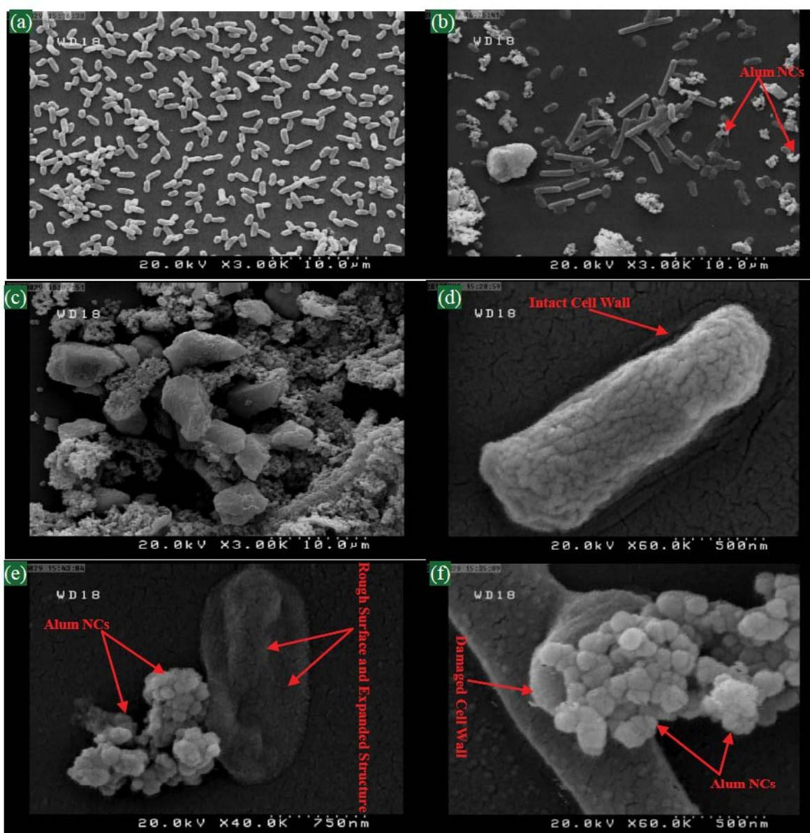
Fig. 5. FE-SEM images of (a and d) *E. coli* (control) and (b, c, e, and f) *E. coli* obtained after 15 and 25 min reaction time with alum NCs.
