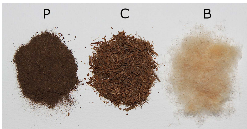
Fig. 1. Materials used in sorption experiments: P – peat; C – coconut; B – broadleaf before mercerization process (Photo: Ciesielczuk T).
