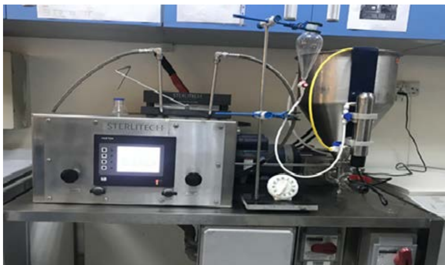
Fig. 1. Lab-scale UV disinfection with UF membrane testing skid.
