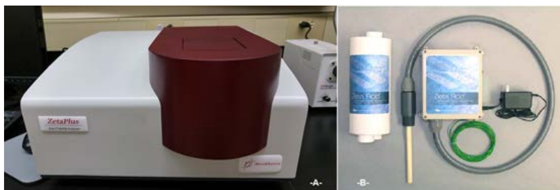
Fig. 2. Zeta plus (a) and zeta rod (b) instruments used to measure and control zeta potential.
