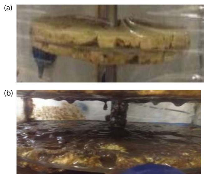
Fig. 2. Rotating biological contactors before the biofilm formation (a) and after biofilm formation in the aeration basin (b).
