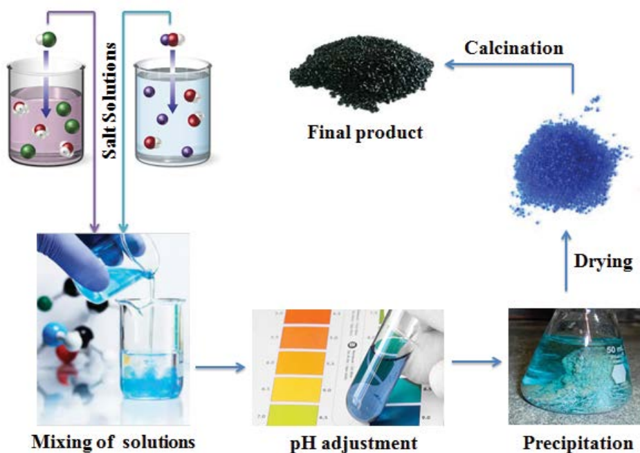
Fig. 1. Schematic illustration of co-precipitation route to synthesize different oxides.
