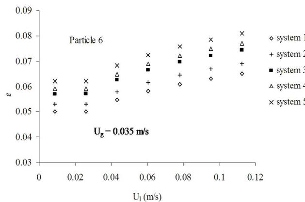
Fig. 4. Effect of physical properties of liquids on bed voidage.
