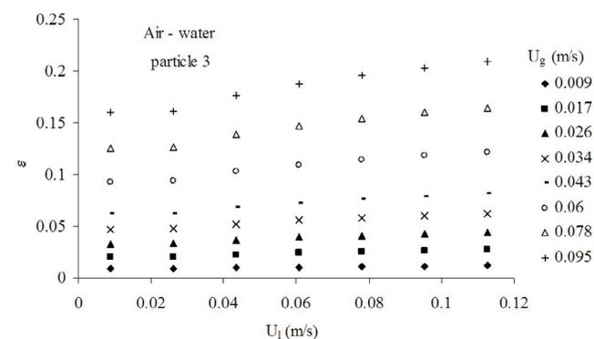
Fig. 1. Effect of liquid and gas velocities on bed voidage.
