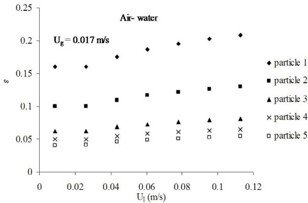
Fig. 2. Effect of particle diameter on bed voidage.
