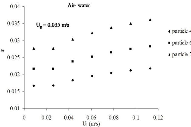
Fig. 3. Effect of sphericity of particle on bed voidage.
