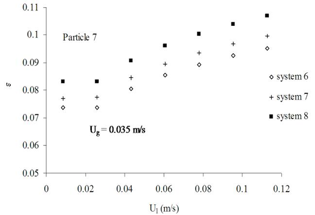
Fig. 5. Effect of rheological properties of non-Newtonian liquids on bed voidage
