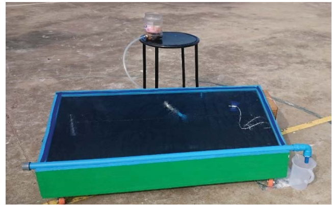
Fig. 1. Single slope basin type passive solar still.
