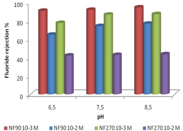
Fig. 5. Evolution of fluoride rejection at different pH and concentration.
