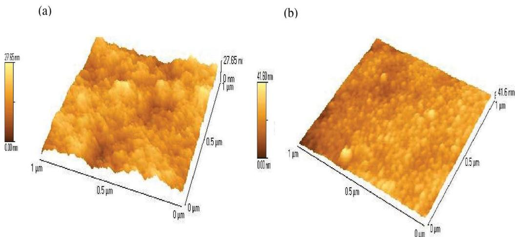
Fig. 3. Three-dimensional AFM images of the surface of (a) NF90, (b) NF270 membranes on a scan area of  $1 \mu\text{m} \times 1 \mu\text{m}$ .
