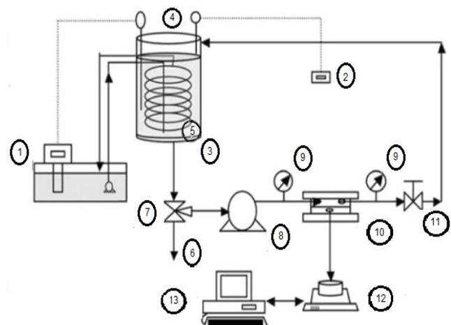
Fig. 1. Schematic experimental setup of the pilot plant with spiral membranes used. (1)-Circulating thermal bath, (2)-preference thermometer, (3)-feed tank, (4)-temperature probe, (5)-coil, (6)-purge, (7)-three-way valve, (8)-high-pressure pump, (9)-manometer, (10)-Sepa CF II Cell, (11)-pressure control valve, (12)-balance, (13)-computer.
