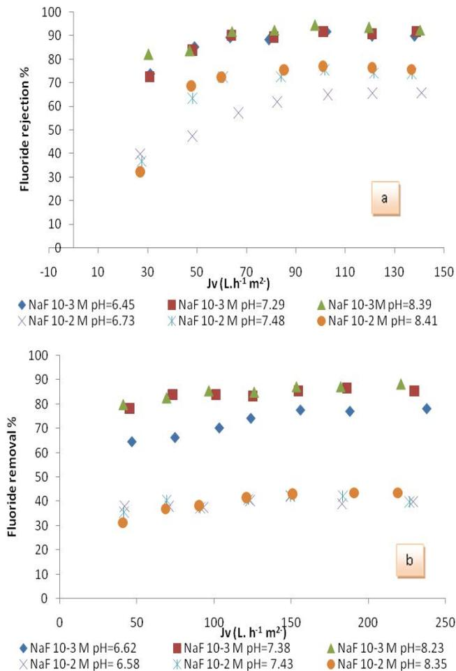
Fig. 4. Variation of fluoride rejection vs. permeate flux for NF90 (a) and NF270 (b).
