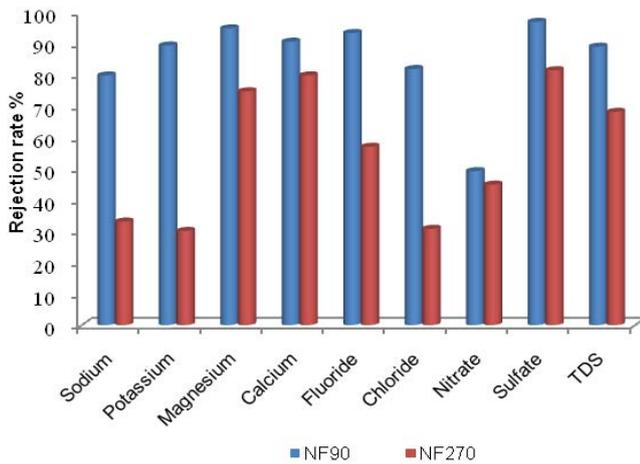
Fig. 6. Average rejection of TDS and common ions in Kouinine feed water by the investigated membranes.
