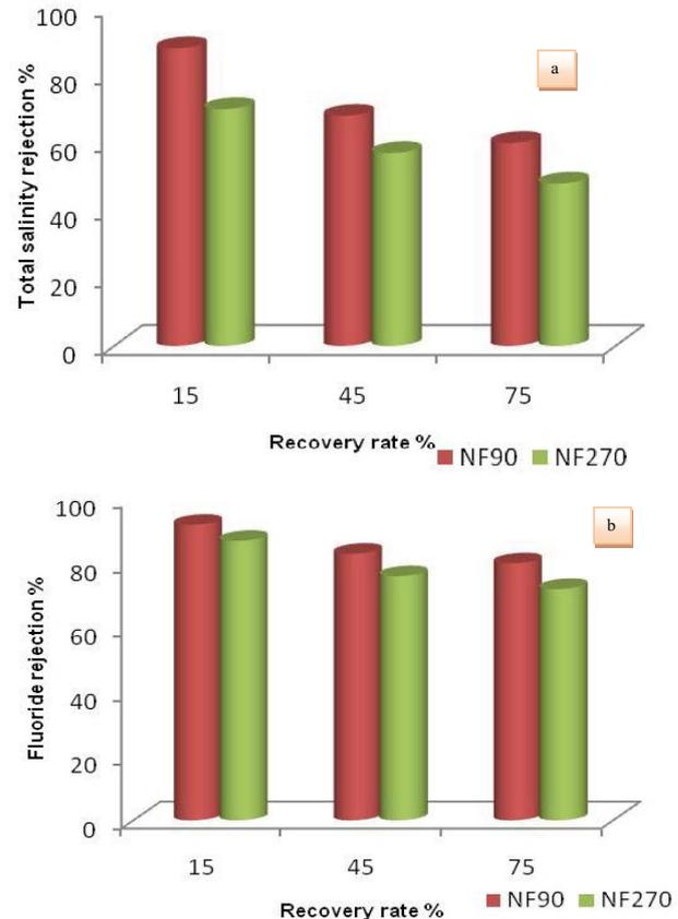
Fig. 7. Total salinity rejection (a) and fluoride rejection (b) during Kouinine water desalination by NF membranes for recovery values of 15%–75%.
