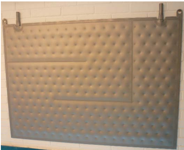
Fig. 1. Plate-type heat exchanger used in the commercial Sulzer static crystalliser.
