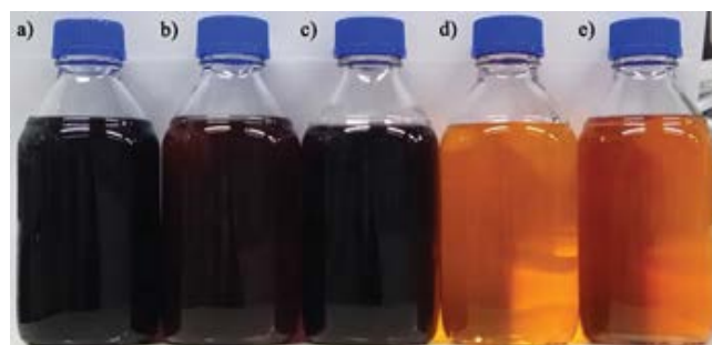
Fig. 2. Comparison of the initial post-fermentation broth (a) and permeates obtained in NF process: (b) 450 Da membrane and TMP = 1.60 MPa, (c) 450 Da membrane and TMP = 1.20 MPa, (d) 200 Da membrane and TMP = 1.60 MPa, and (e) 200 Da membrane and TMP = 1.20 MPa.
