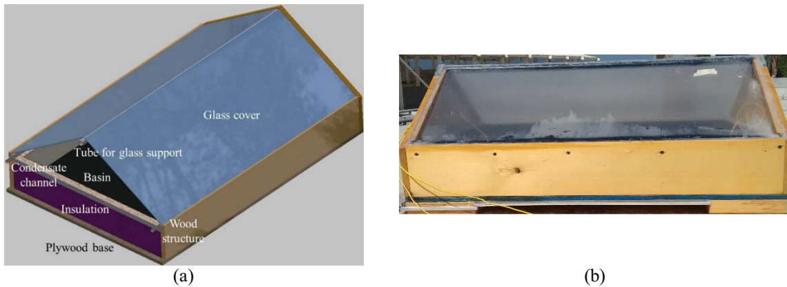
Fig. 2. 3D view of the solar still assembly (a), and side view of the solar still in operation (b).
